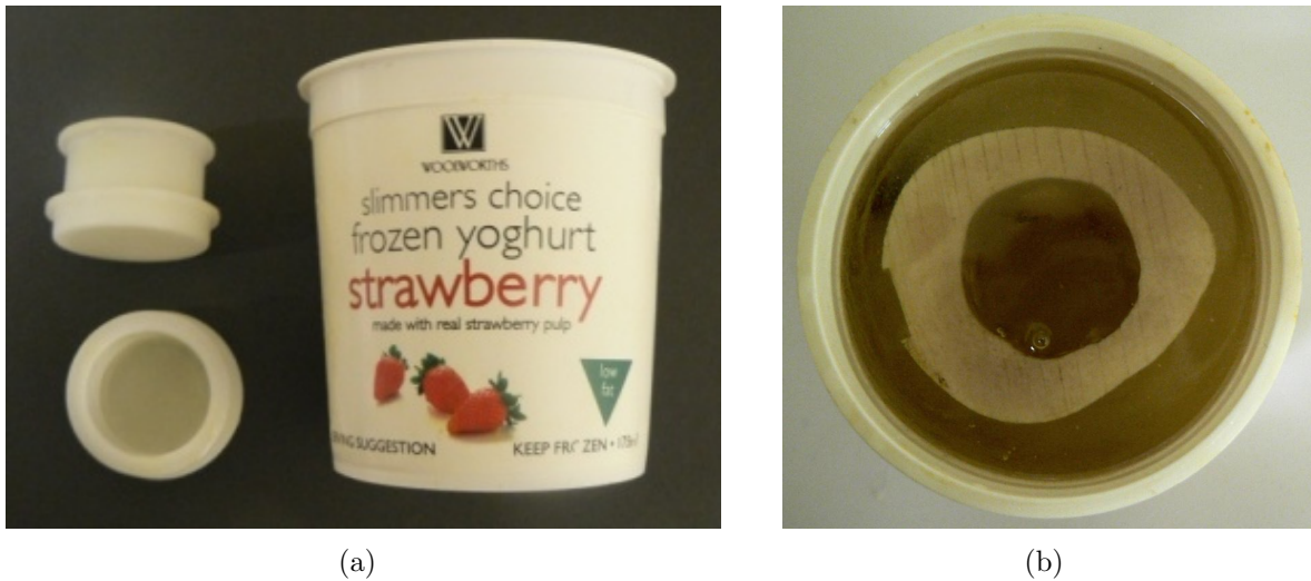
Figure 3.5: Photographs of (a) suitable containers for specimen embedding: custom moulds with removable bases and a yoghurt container and (b) a bone diaphysis specimen embedded in resin inside a container of the right size.
