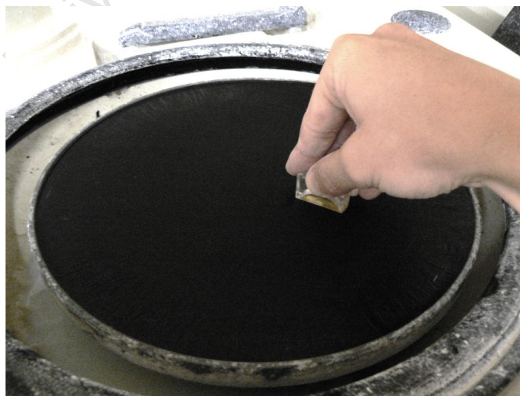
Figure 3.7: A photograph of the final polishing of a specimen with an Op-Chem polishing cloth on a lap wheel
