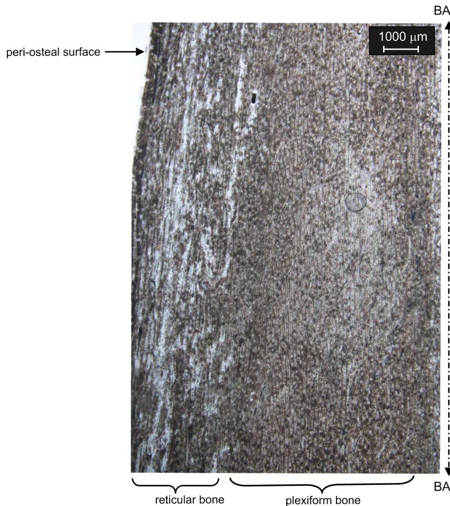
Figure 3.17: A micrograph of a longitudinal section of a bovine femur diaphysis
