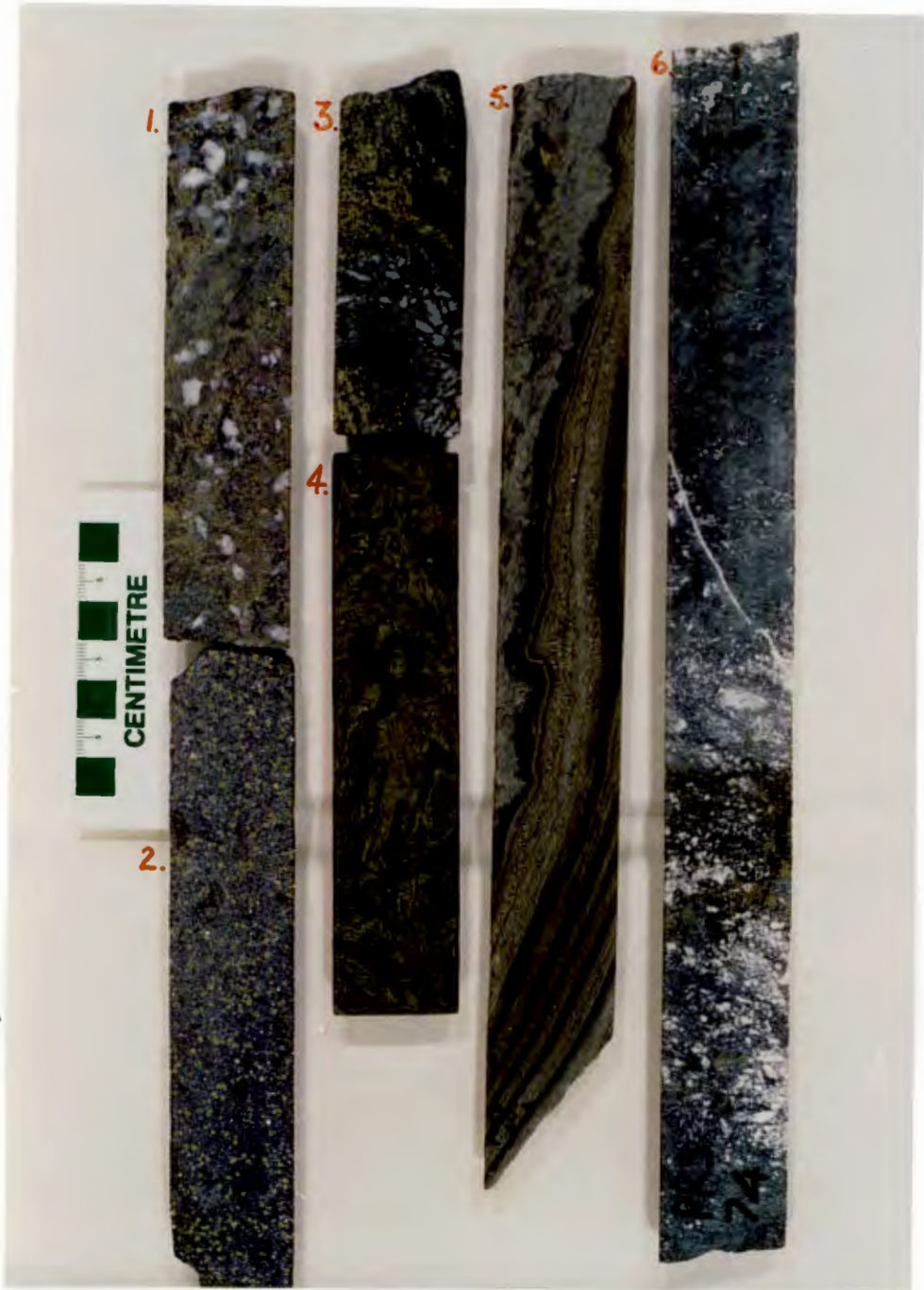
Plate 4: Textures of ore zone lithologies. (1,2) Massive sulphide ore. (3) Laths of barium carbonate are hosted by dolomite. (4) Soft sediment deformation in mixed sulphide-argillite layers. (5) Density bedded silica-barite rock with evidence of flame structures and density contrasts. (6) Typical dolomite ore with blebs and laths of barium carbonate .
