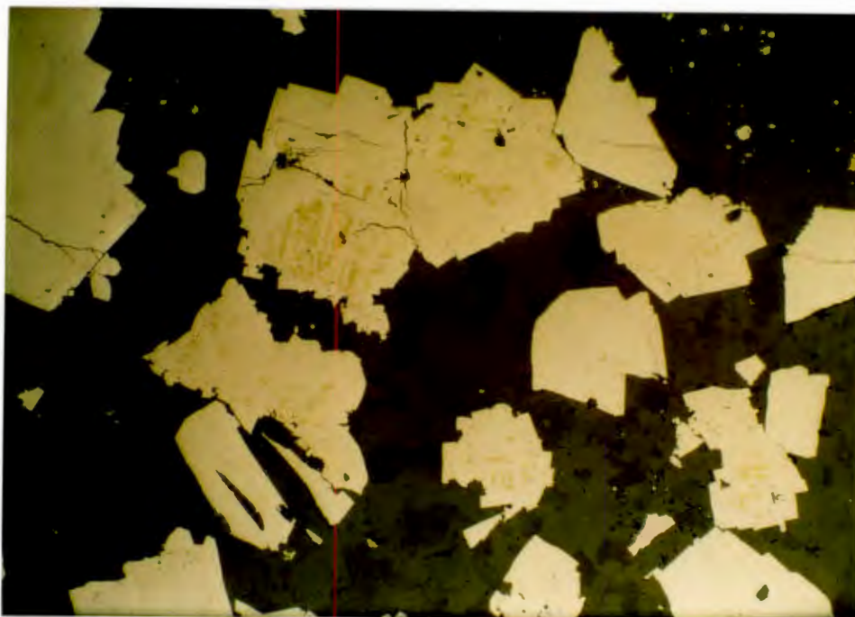
Plate 7: Angular pyrite present in type 3 sulphide veins. Cruciform chalcopyrite replacement can be noticed. PRS 95, X.40
