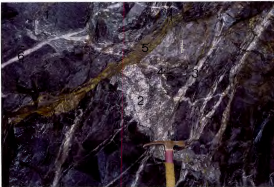
Plate 30: Multiple vein assemblage in footwall quartzites. Bedding is roughly horizontal while type 1 carbonate veins and spots are present. Veins are identified as follows: 1. Irregular type 3 carbonate (D1 in age), 2. Type 4 carbonate vein (early D2 in age), 3. irregular quartz + baryto-calcite vein (D2), 4. type 3 sulphide vein (late D2) and 5. type 4 quartz vein. Locality MOB [470Ch].
