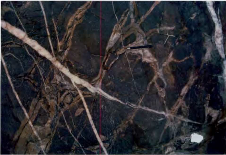
Plate 18: Typical fracture breccia exposed on surface. Crosscutting quartz veins are related to late D2 faulting. Locality 100 m south of A-Mine.
