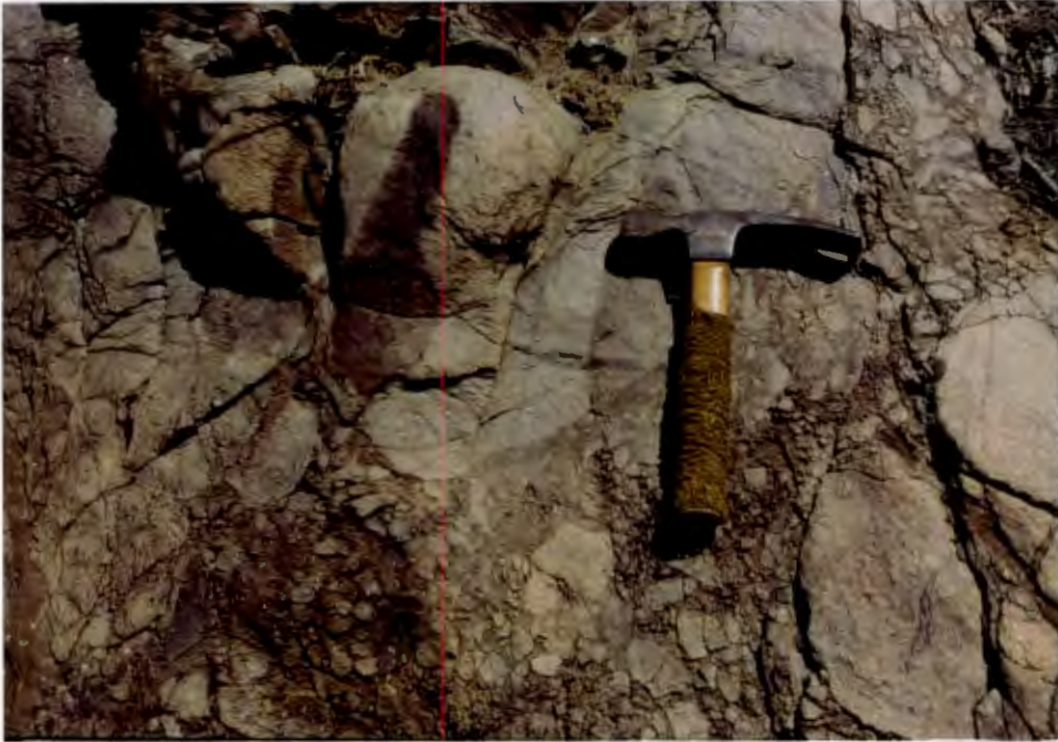
Plate 2: Hydrothermal matrix breccia with evidence of early incomplete silicification as well as heterolithic clast assemblage. Locality MOB surface exposure.
