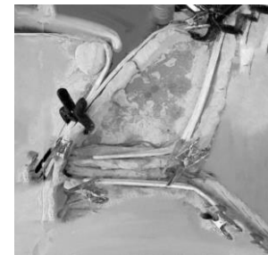
Clamping along clay jig
