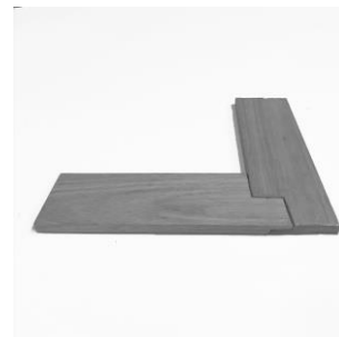
Half Lap x Tongue and Groove Joint
