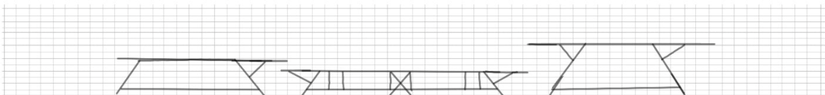
Frame construction extended to roof and plinth, roof infers continuity and interest through staggering and overlap
