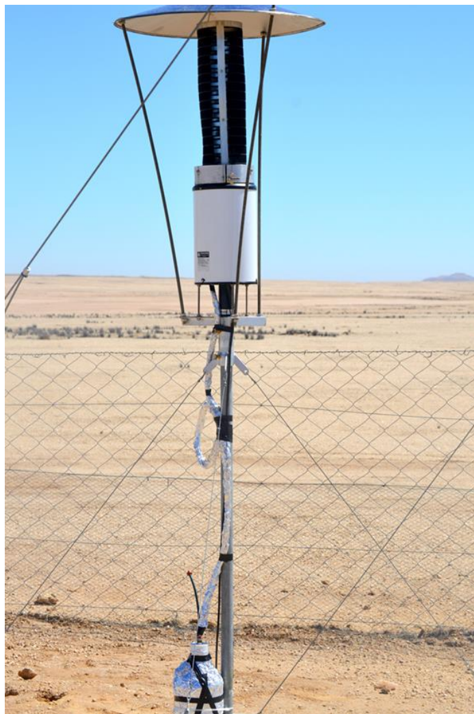
Figure 3.5: Schematic of the set-up of the Juvik fog gauge (Juvik and Ekern, 1978) and one of the gauges ( set up at 1.2 m above ground) at the stations.
