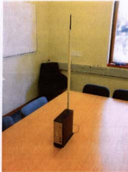
Figure 5.1: Wireless client node with a raised antenna.
