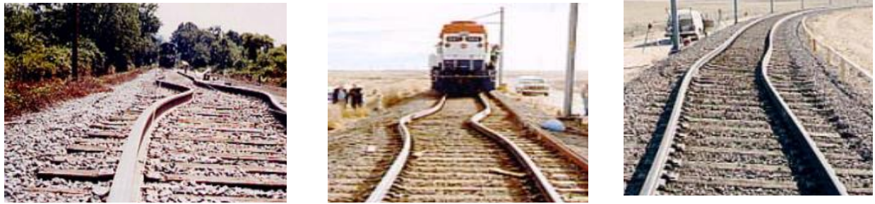
Figure 2.8: Rail buckling illustration (Kish & Mui, 2003)
