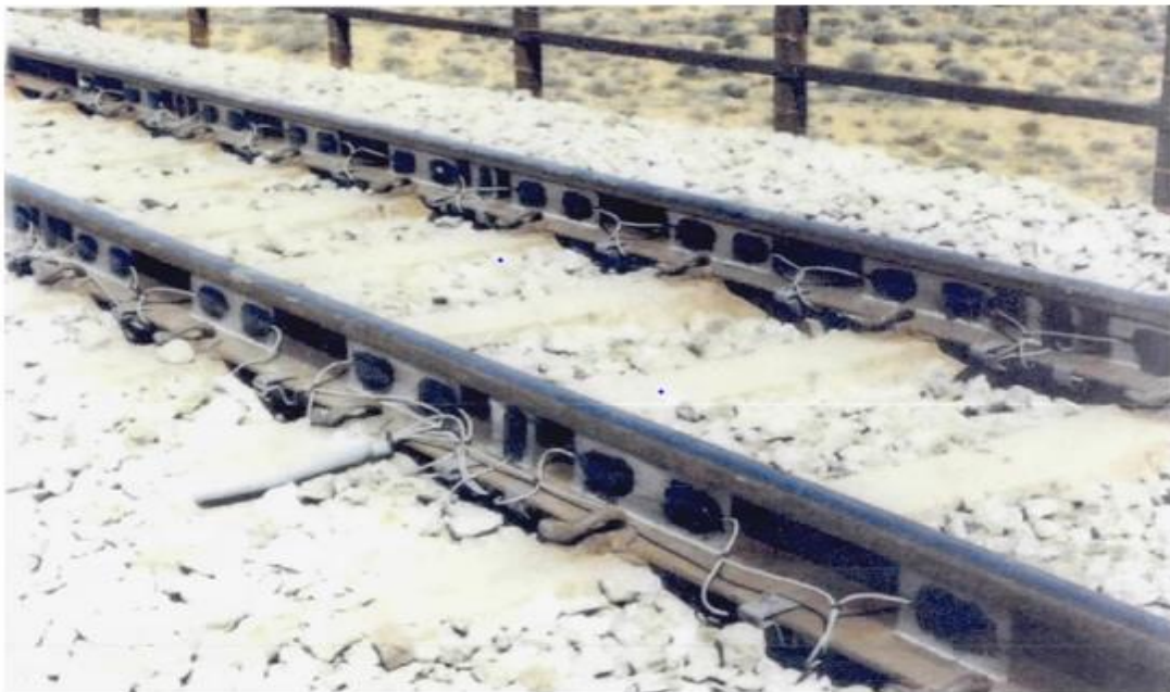
Figure 3.4: Typical WIM-WIM sensors
