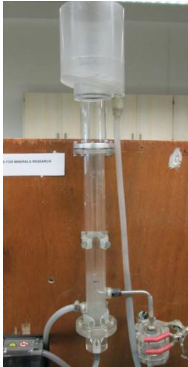
Figure 3.3: Bench-scale flotation column
