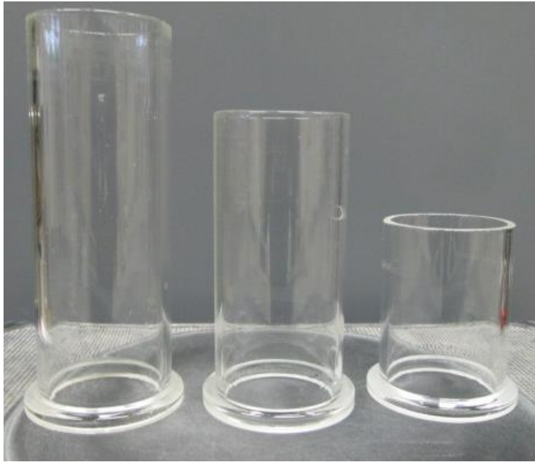
(b) The three glass columns; from left to right: 11, 7, and 4 cm height
