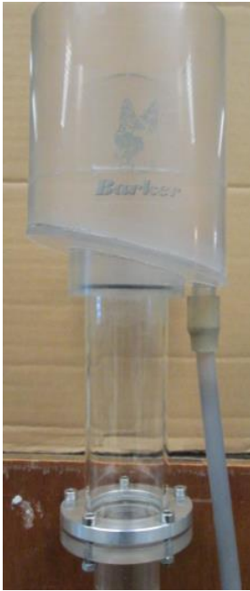
(a) Froth section of flotation column
