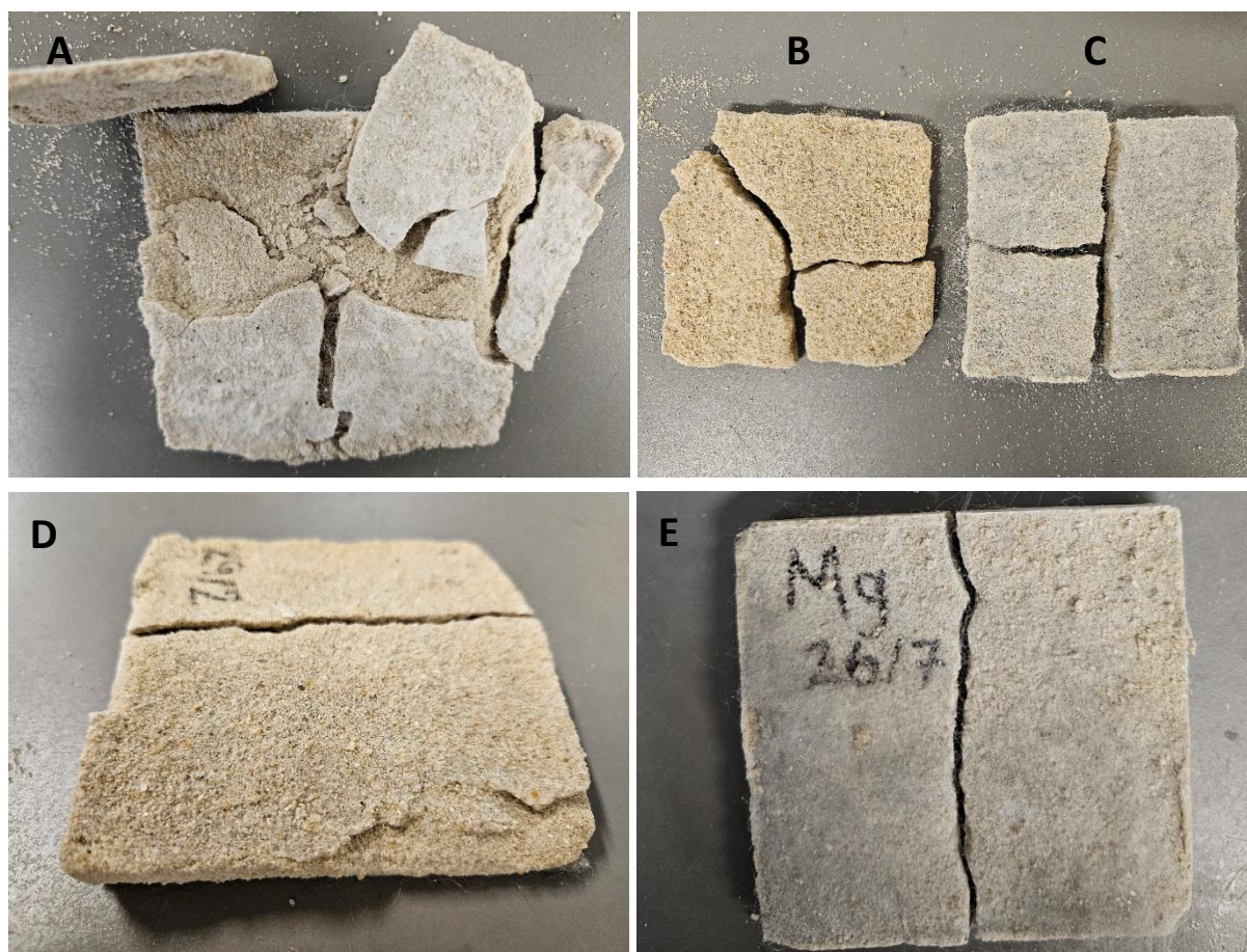
Figure 7.5: Bio-tiles (roughly 100 x 100 mm) grown with liquid bacteria solution (A) instead of bio-slurry, a daily nutrient broth-enriched treatment and no additional \text{CaCO}_3 seeds (B and C) compared to a bio-tile grown with nutrient broth and additional seeds (D), and a bio-tile grown with nutrient broth and additional seeds and magnesium (E). All bio-tiles are cracked because the picture was taken after determining the breaking strength.
