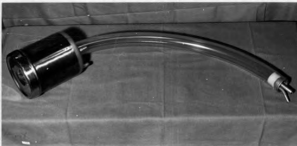
Debubbling system: the mixing tube shown after insertion into the bottom of the can. The two peripherally placed outlets can be seen.
