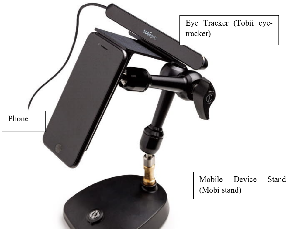
Figure 10: Experimental Eye-Tracking Set-up
