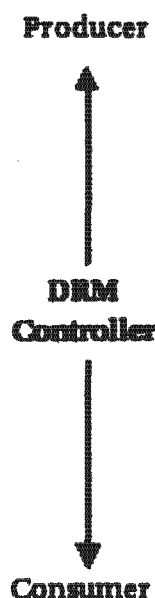
Figure 12.1: Web of Trust with only the DRM Controller
