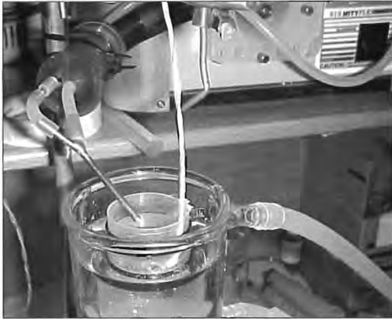
Figure 8-1 Picture of Fluid Dispenser Configuration, showing the receptacle with the dispenser delivery pipe just inside it and the glass cup-horn containing the transmitting fluid (in this case water).
