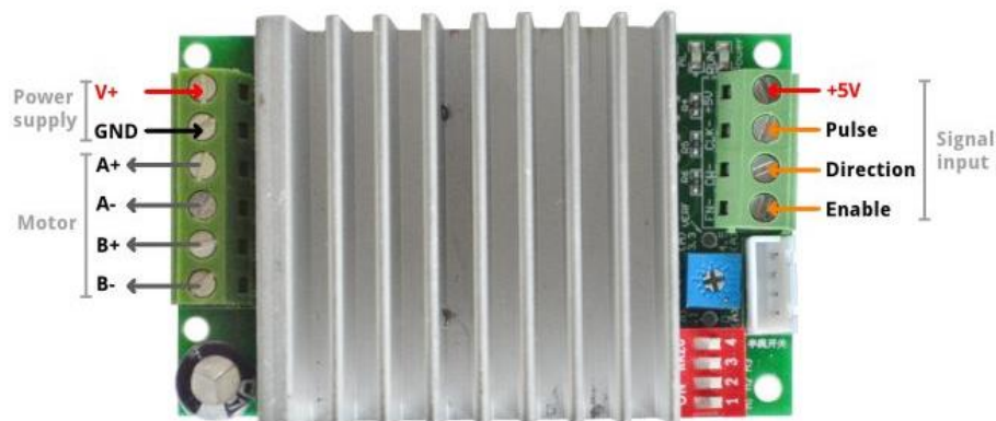
Figure 3-27 TB6600 Wiring scheme for connection to the power supply and the stepper motor.
