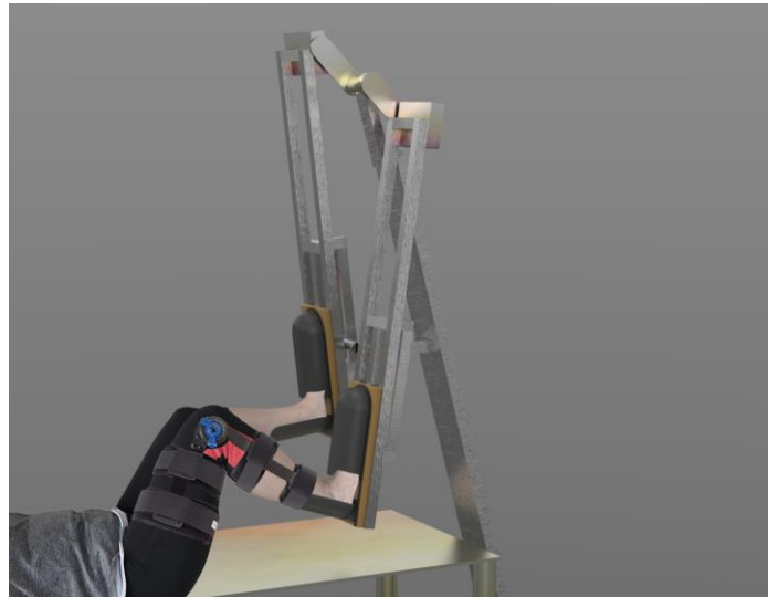
Figure 6-1 Possible implementation of a knee brace to reduce rotational movement of the legs.
