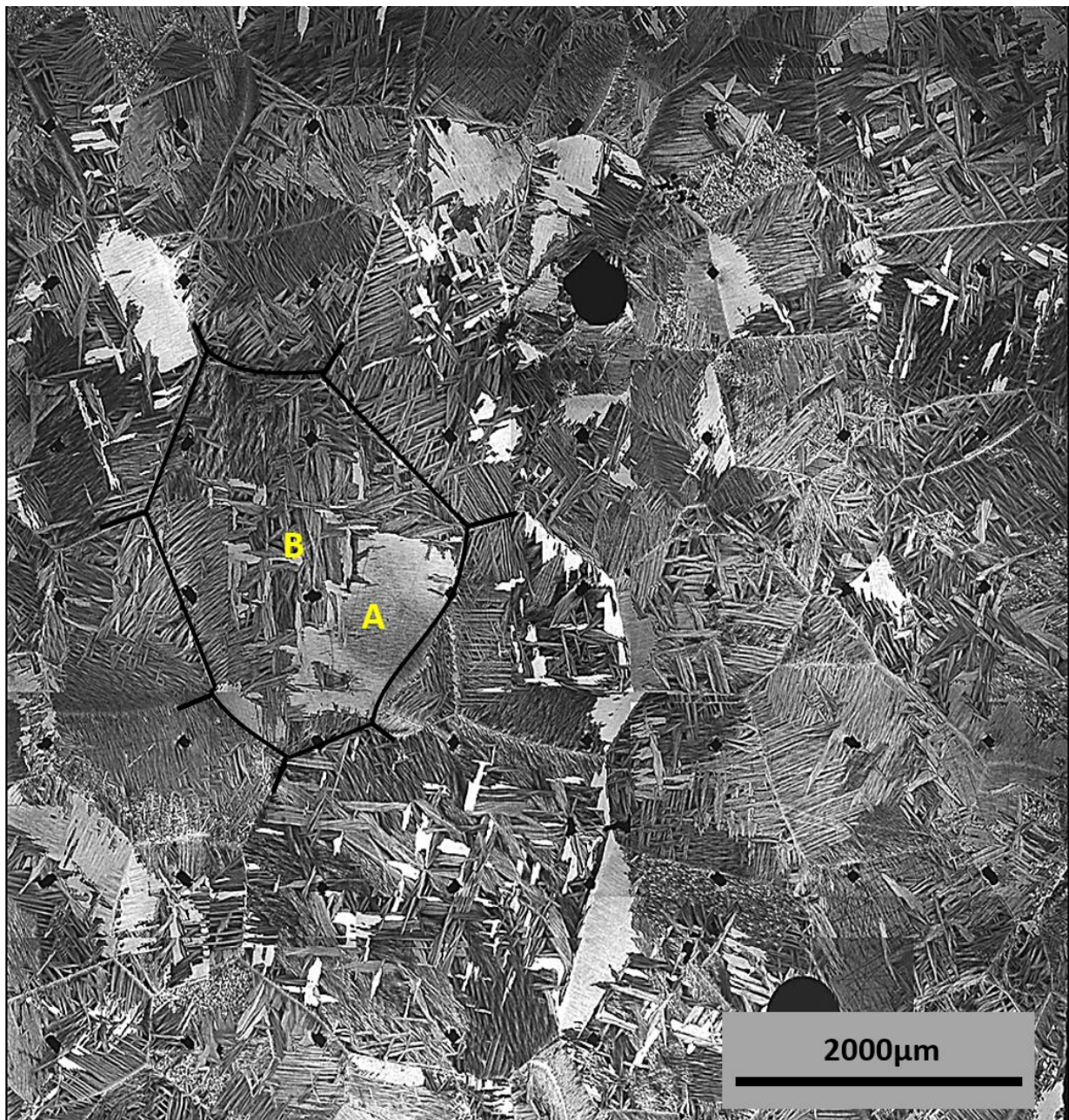
Figure 1. 2: The as-cast microstructure forms when slow cooling molten Ti-6Al-4V to room temperature. It has coarse prior beta grain sizes of up to 2000 \mu\text{m} diameter (highlighted in black) Widmanstätten (A) and basketweave morphologies (B). The micrograph also shows a network of 1mm spaced hardness indents and porosity in the as-cast microstructure. 3
