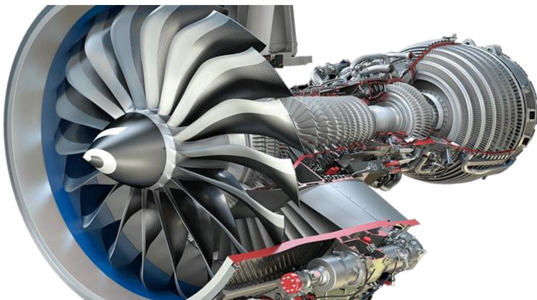
Figure 1. 1: The CFM International LEAP aircraft engine which incorporates titanium castings. 2
