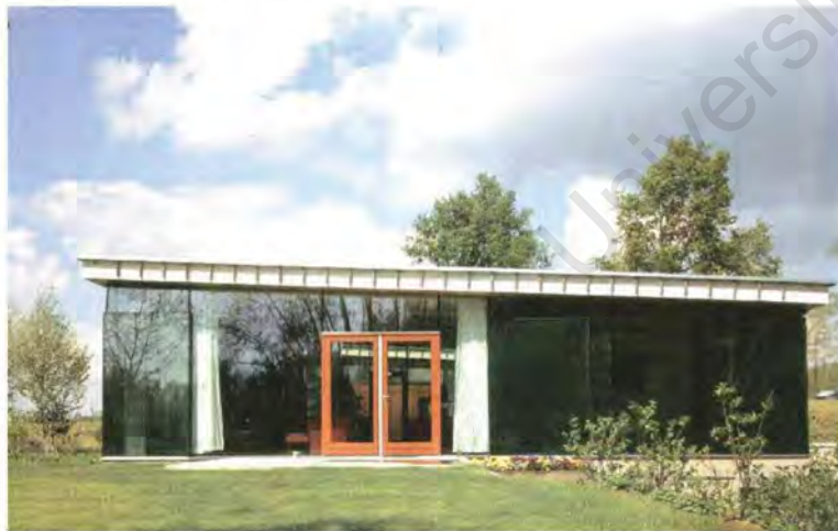
Fig 66 Laminata House exterior has vertical stacked glass sheet structural walls, Interior quality of light, vertically stacked glass sheet walls [Richards, 2006:194]
