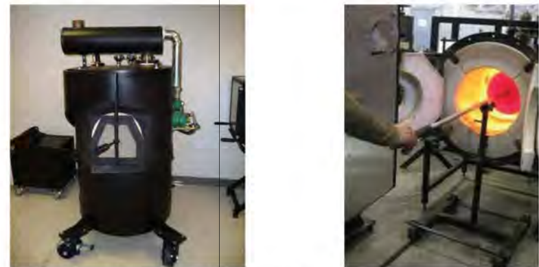
Figure 86 Modern Glass Melting furnaces use gas or electricity [www.cmog.org, 2013]
