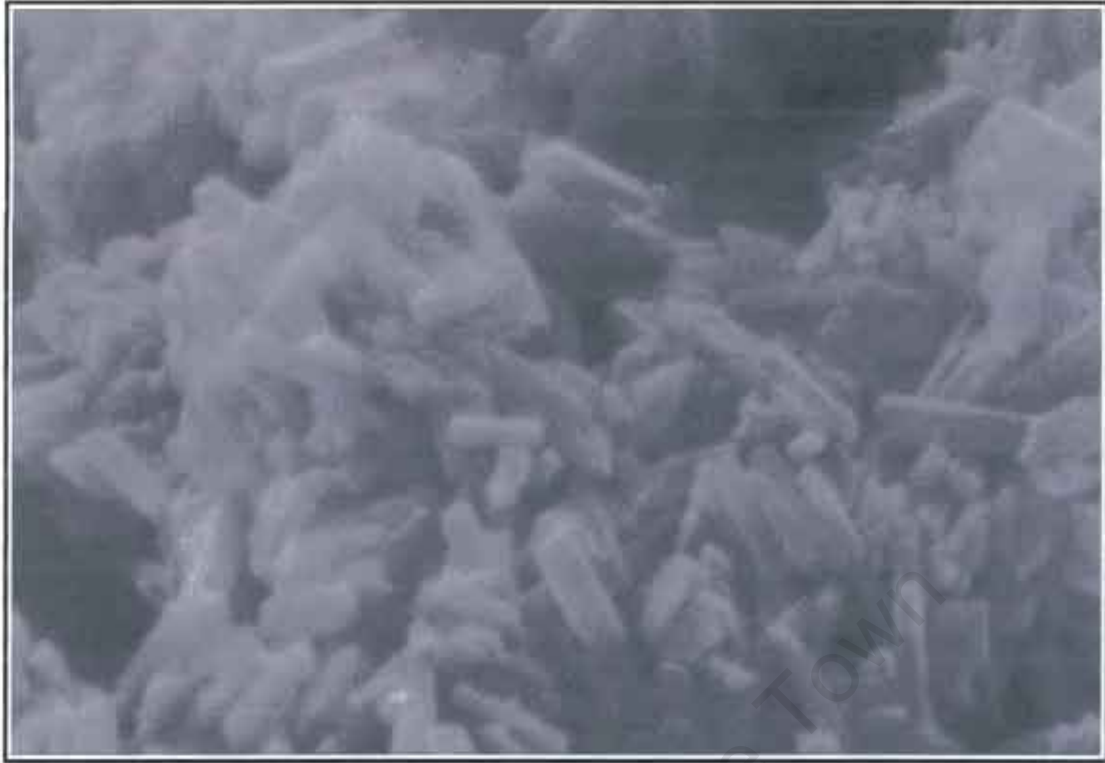
Plate 6.1: Scanning electron micrograph of synthetic \beta -haematin. Synthesised according to the method of Egan et al (Egan et al. , 1999a), (magnification: x 50 000)
