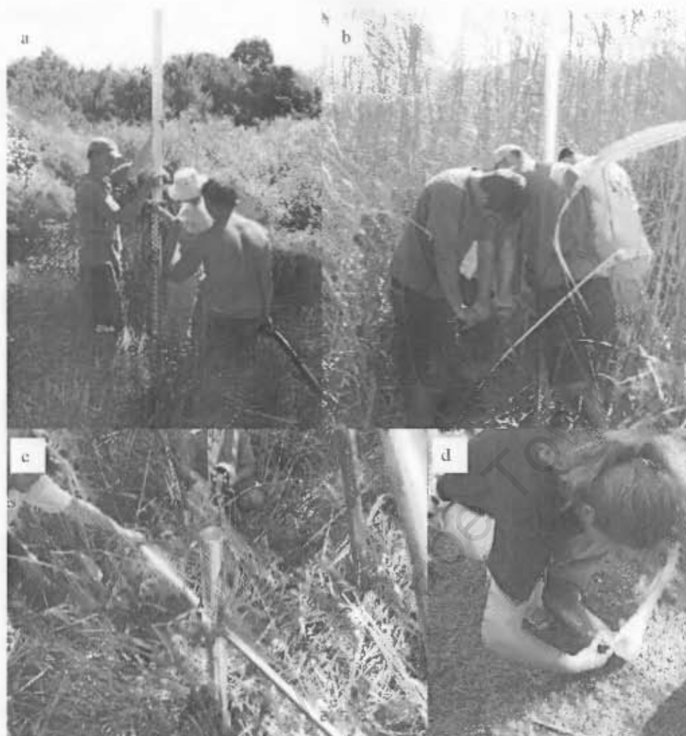
Figure 14: The vibracoring process a) equipment set-up; b) pushing core down into the sediment; c) wrenching core out using a tripod and d) sealing and labelling cores
