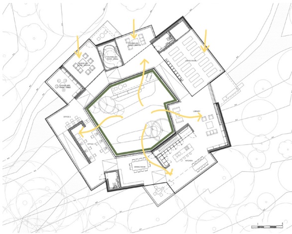
Figure 28: Glasgow Floor plan showing access to courtyard and natural light.
