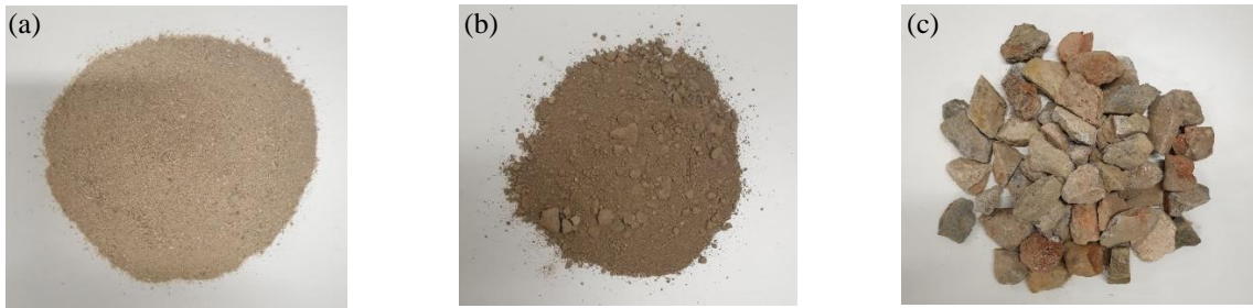
Figure 3-5: Geomaterials; (a) Sand, (b) Gravelly Sand & (c) Leachate Collection Stone
