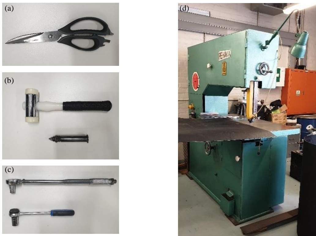
Figure 3-9: Geosynthetic preparation tools; (a) A pair of scissors, (b) Hammer and puncher, (c) Ratchet, & (d) Mechanical saw machine
