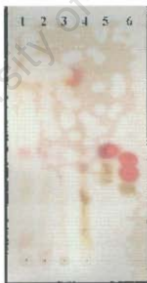
Fig. 4. Separation of whole-cell sugars from actinomycete hydrolysates by thin-layer chromatography. 1. P 1 m 2. O 1 o 3. SS12 4. R 2 μ 5. Ribose-Mannose-Glucose standard 6. Xylose-Arabinose-Galactose standard. Order of sugars in standards as seen from top to bottom.
