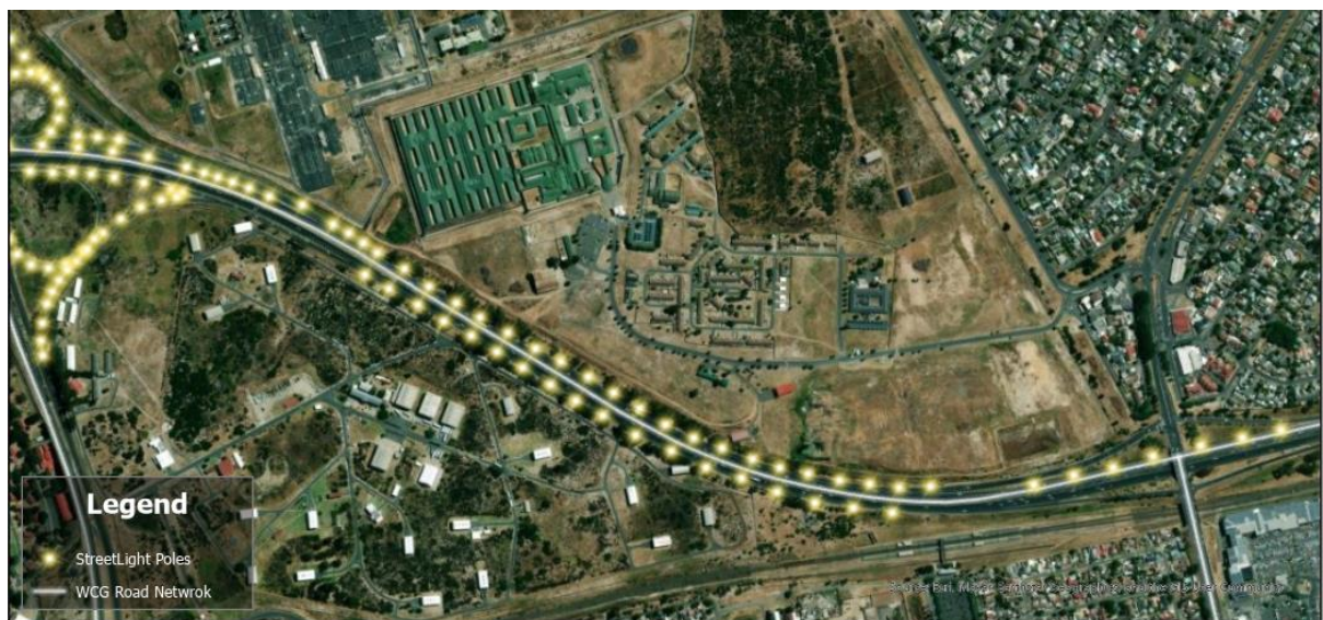
Figure 23: Streetlight spacing on the N1
