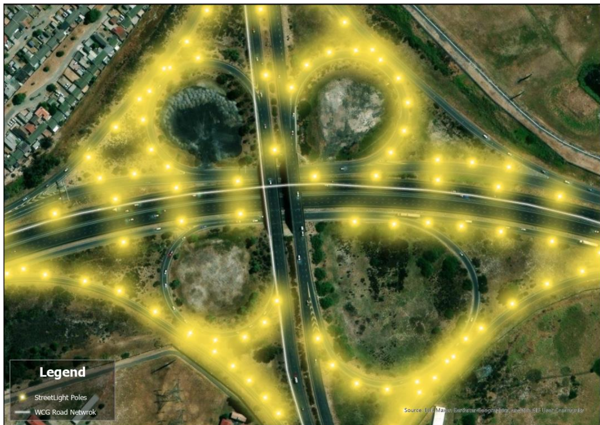
Figure 22: Streetlights in the N7 and N1 interchange
