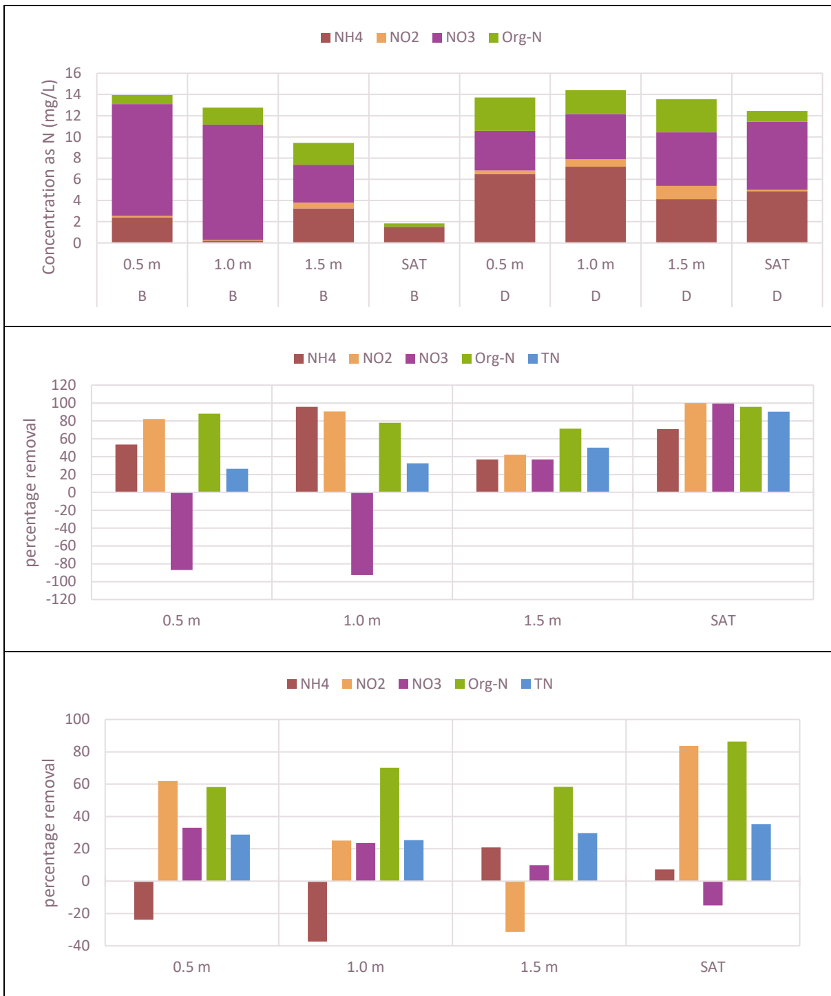
Figure 5-15: Nitrogen species concentration in Experiments B and D (top), percentage removals in Experiment B (middle) and in Experiment D (bottom).
