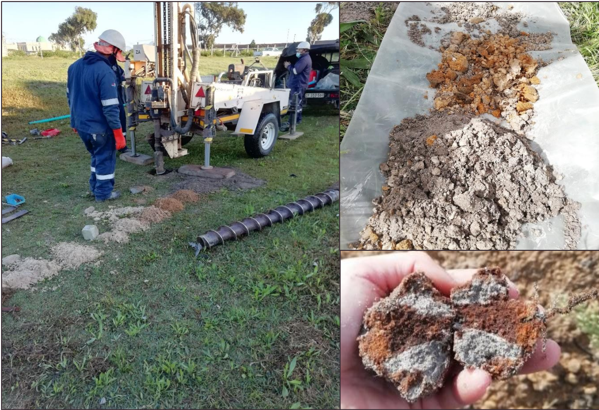
Figure 4-3: Soils encountered during drilling at position 1 (left) position 3 (top right) and mottles in soft soil ped (bottom right).
