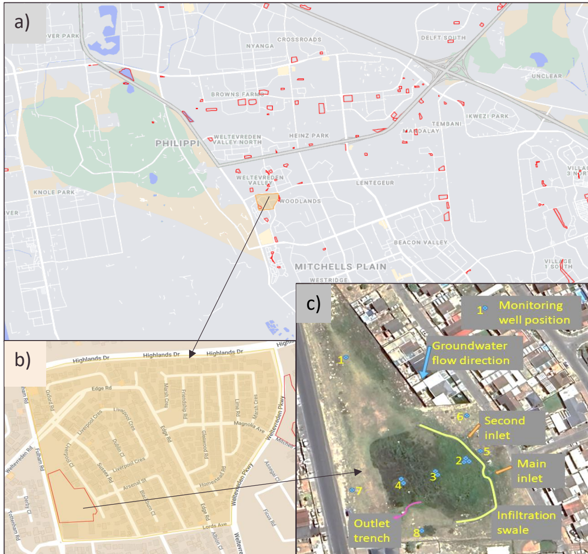
Figure 4-2: a) Location of the study site in Mitchell's Plain with stormwater ponds in red; b) map of the local catchment area (gold polygon) and study site (red outline); and c) Study site layout (Image source: Google, 2023).
