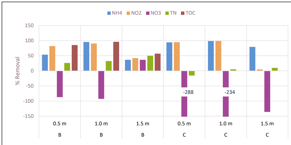
Figure 5-8: Percent removals of nitrogen species and TOC during infiltration with (B) and without (C) organic carbon in SSW.
