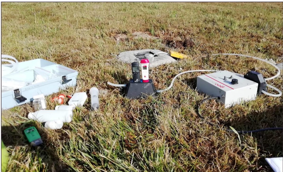
Figure 4-9: Low flow groundwater sampling set-up.
