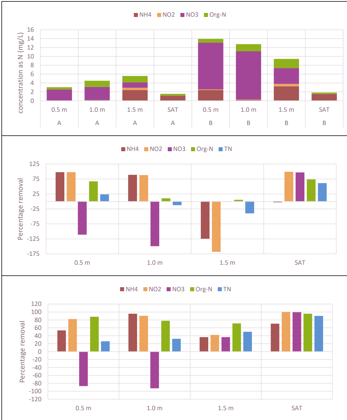
Figure 5-14: Nitrogen species concentration in Experiments A and B (top), percentage removals in Experiment A (middle) and in Experiment B (bottom).
