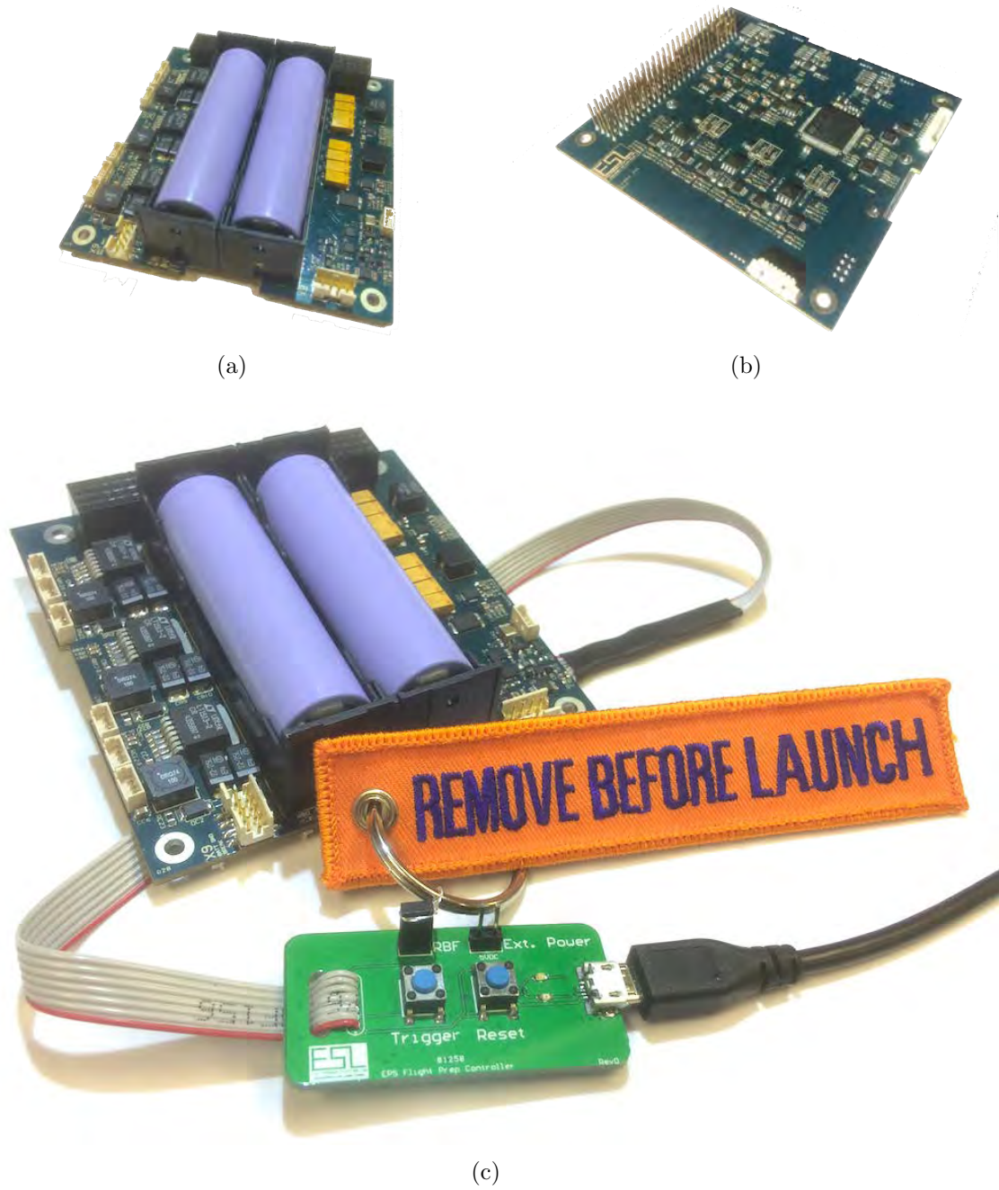
Figure A.5: Photographs of the prototype module. (a) Top view, (b) bottom view, and (c) the module with flight controller interface attached.
