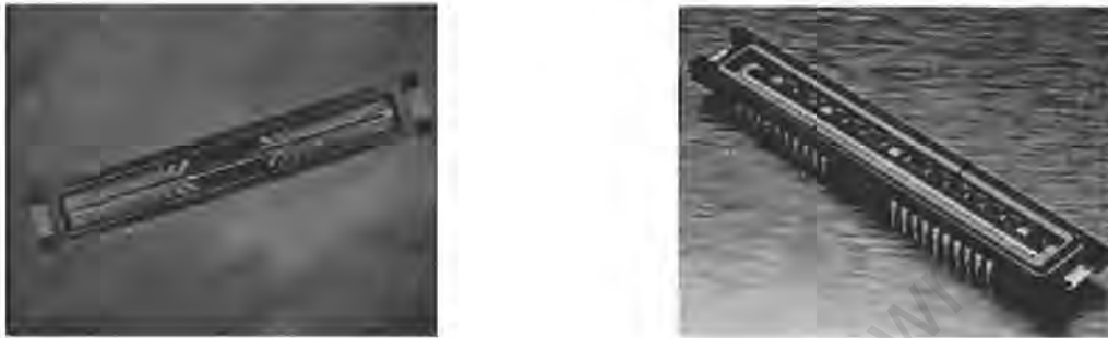
Figure 3.2 Colour and monochrome linear sensors from Kodak. Colour linear CCD sensor KLI-14403 with 14 403x3 (RGB) pixels, 72 mm long with pixel size 5 x 5 \mu\text{m} (left) and monochrome linear CCD sensor KLI-8811 with 8800 pixels, 61.3 mm long with pixel size 7 x 7 \mu\text{m} (right).
