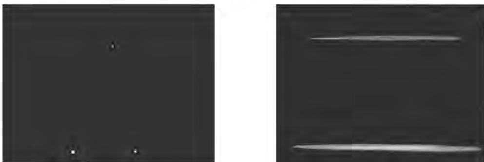
Figure 5.8 Calibration frame consisting of 19 active targets with 3 of them switched on (left) and their image on the camera where the light is converted by the cylindrical lens (right).
