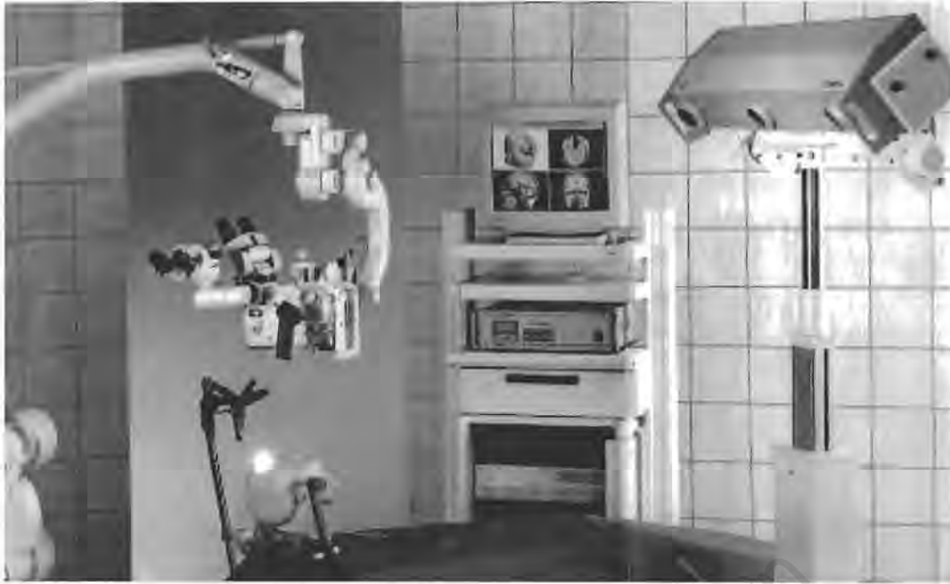
Figure 7.7 ViewScope neuro-navigational system (Elekta, Stockholm, Sweden) consisting of a surgical microscope from Leica (left) optical tracking localizer OPTOTRAK 3000 (right) and the image processing and visualization unit (middle).
