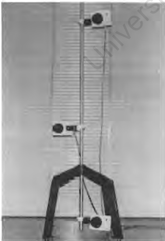
Figure 2.7 Positioning of the camera in the stereometric unit used by Bianchi et al. (1990).
