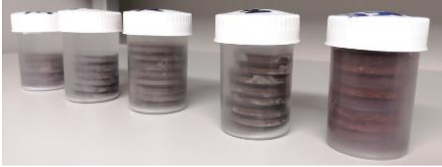
Figure 3.7: Storage of paste specimens for TGA and XRD
