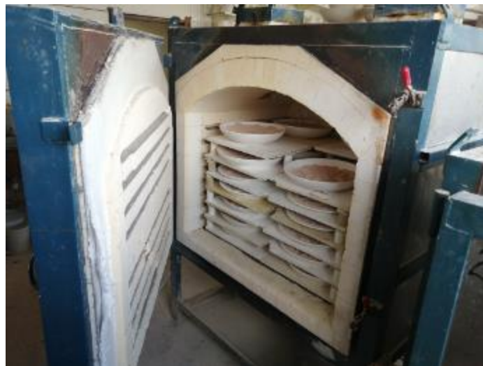
Figure 3.3: Kiln used to calcine sample of clays, also showing the clay bowls containing the clays to be calcined.
