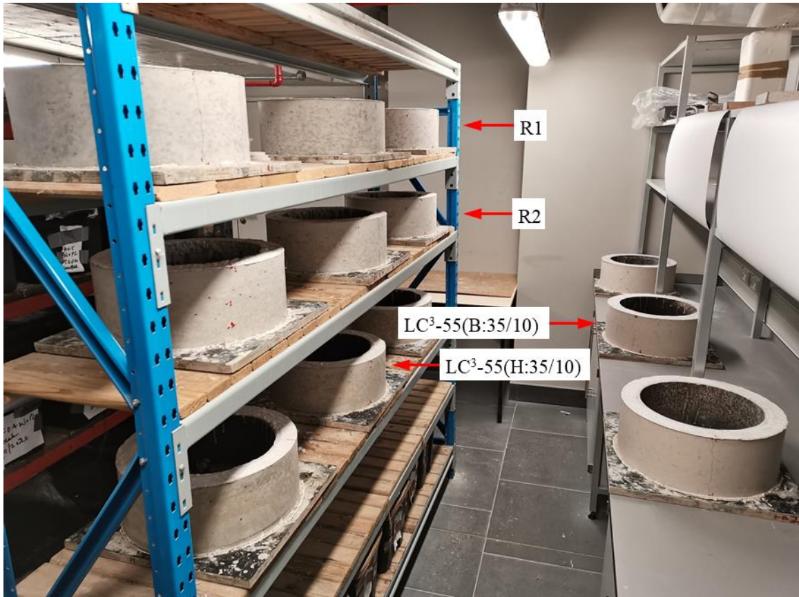
Figure 3.12: Concrete ring specimens
