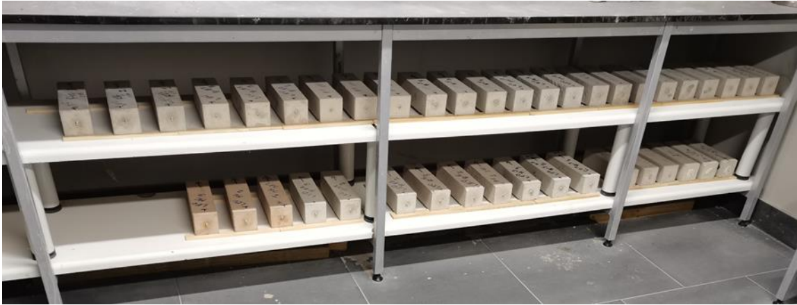
Figure 3.9: Free shrinkage specimens
