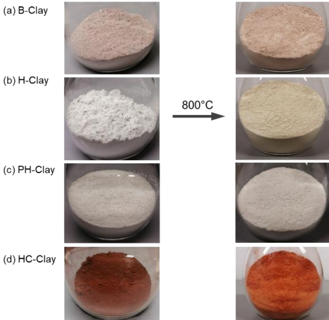
Figure 4.3: Photos of the samples of clays, before (left) and after (right) calcination
