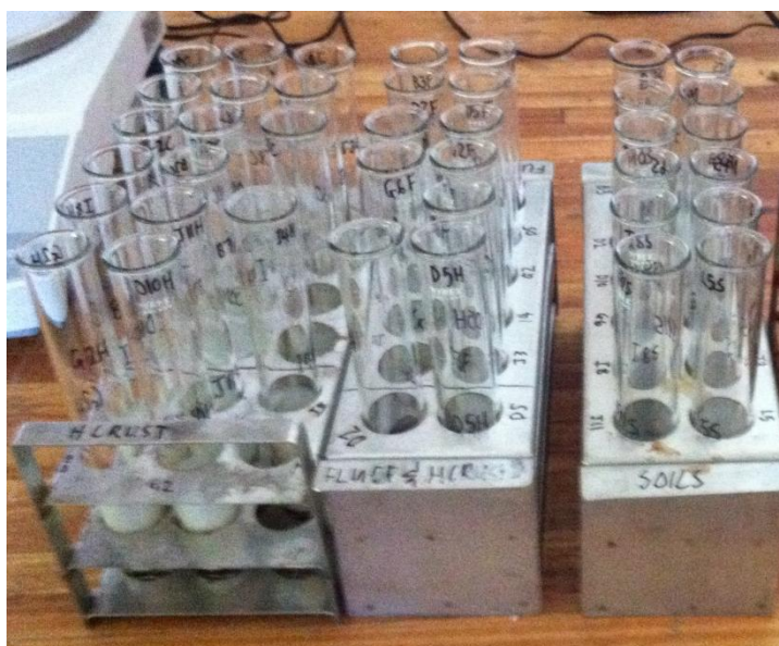
Figure A 3.1 Pre-labelled and weighed glass test tubes with samples following the loss of organics in preparation for drying.
