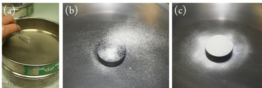
Figure A 7.2 (a) screening the sample onto the disc, (b) insufficient coverage, (c) total coverage of disc before mechanical removal using compressed air.
