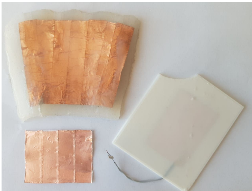
Figure 3.6: Image of Custom Capacitive Sensors Made with Copper Tape. Bottom Left: Sensor Without Embedding, Far Right: Sensor Embedded in 3D Printed Material, Top Left: Sensor Embedded in Silicone.
