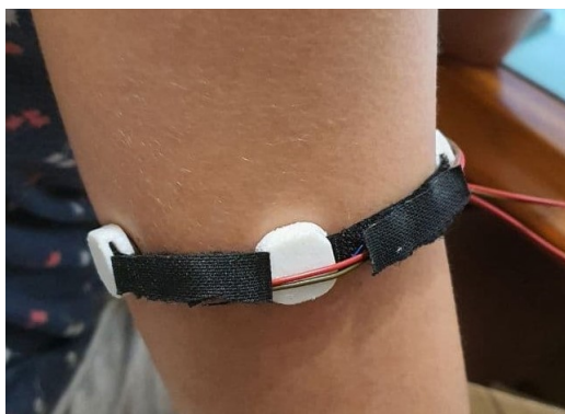
Figure 3.23: Vibrotactile Armband on Participant Upper Arm.
