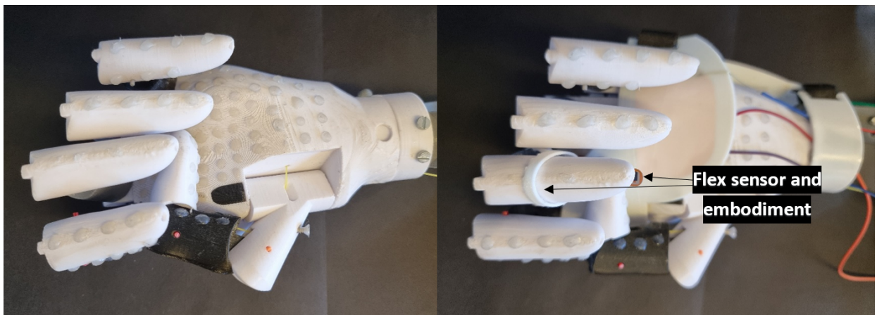
Figure 3.20: Finger Extension of Prosthesis without Flex Sensor Embodiment (Left) and with Flex Sensor Embodiment (Right).
