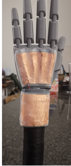
Figure 3.27: Capacitive Sensors Embedded within Silicone Placed on the 3D Printed Static Prosthetic Hand.
