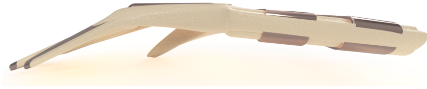
Figure 3.13: CAD Image of the Concept for a Silicone Glove (Capacitive Sensors in Copper) (Side View).
