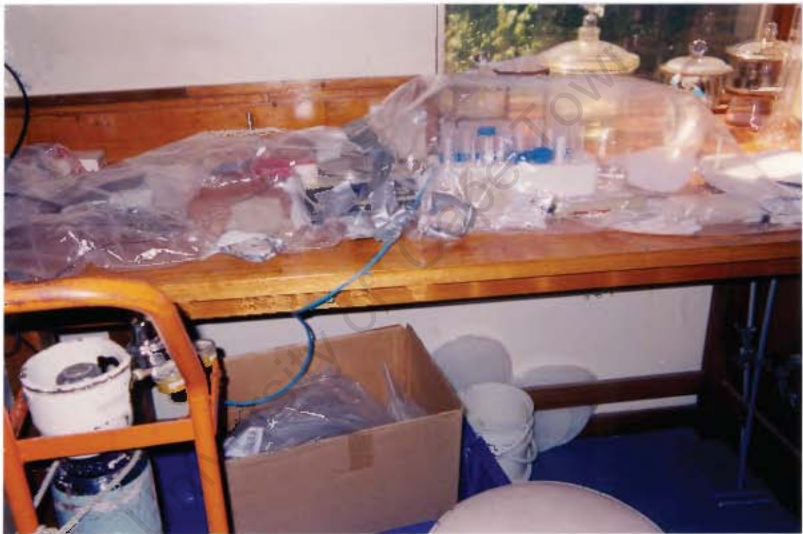
Photo 1: Centrifuge vials in nitrogen bag, made of plastic and duct tape. The bag was filled through a plastic tube inlet, attached to a nitrogen gas canister.
