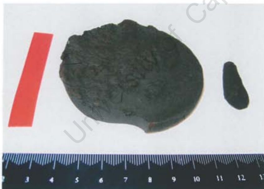
Figure 7.16 The sludge obtained from the SVI measurement for Exp 7.3 dried into a hard cake after ~20 days. Scale in cm.
