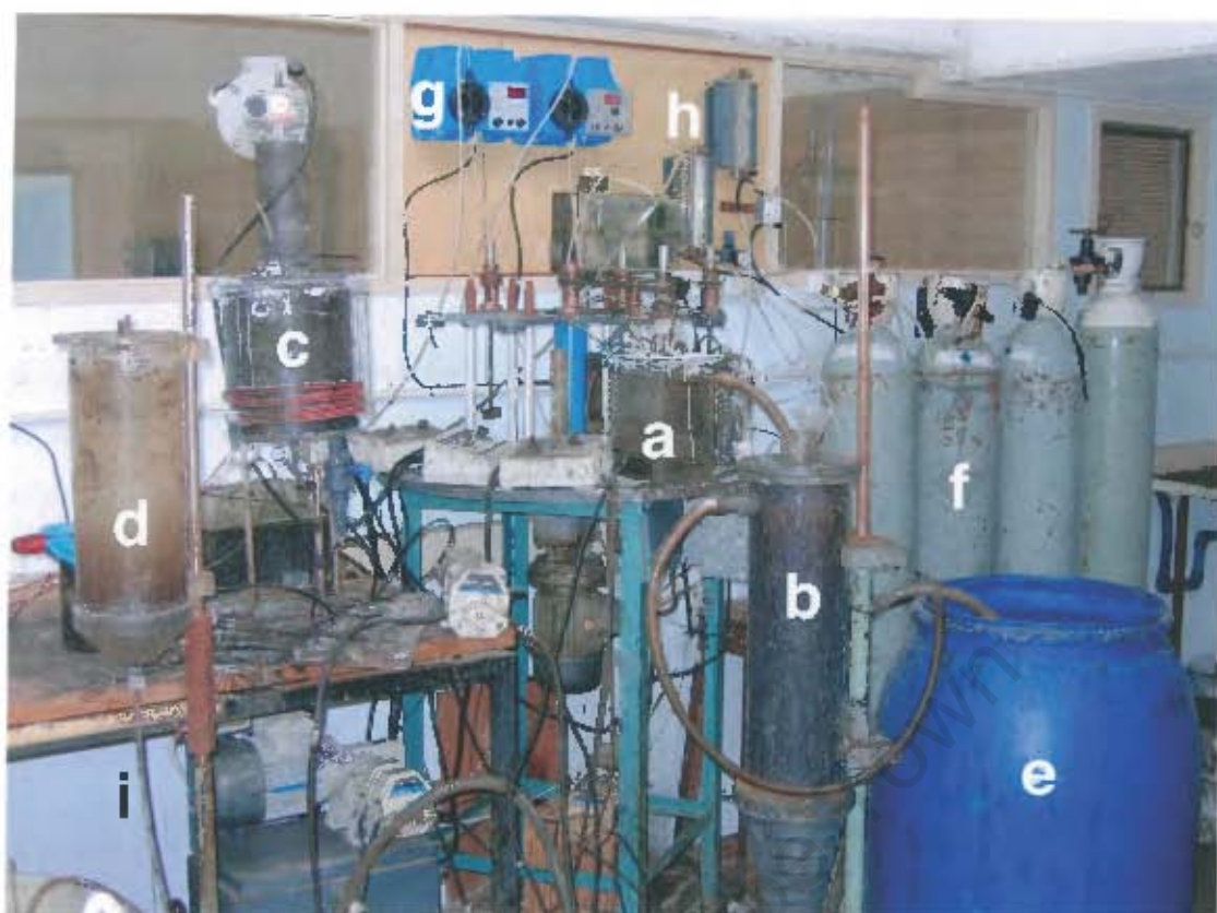
Figure 6.2b Photograph of the apparatus depicted in Figure 6.2a which was used for experiments where calcium was present. a. Contact stabilisation reactor. b. Settler 1. c. Oxidation reactor 1. d. Settler 2. e. Tank receiving effluent from Settler 1. f. Source of air. g. pH controllers. h. Rotameter airflow rate controllers. i. Sludge underflow from Settler 2 to Aging tank (Aging tank and Oxidation reactor 2 not shown)
