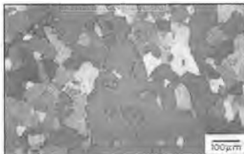
Figure 3.10: Sample ALU2 showing large central cube grain within smaller non-cube grains.
