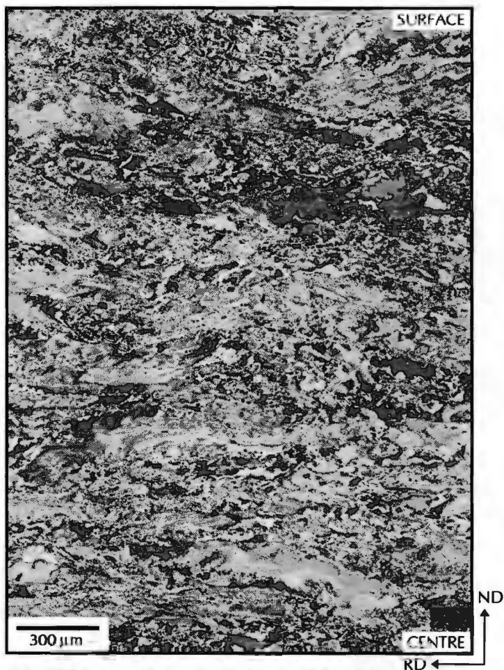
Figure 5.3: ECC image of sample B1, Hot roll finish temperature 920°C. Hot Rolled - Annealed Condition
