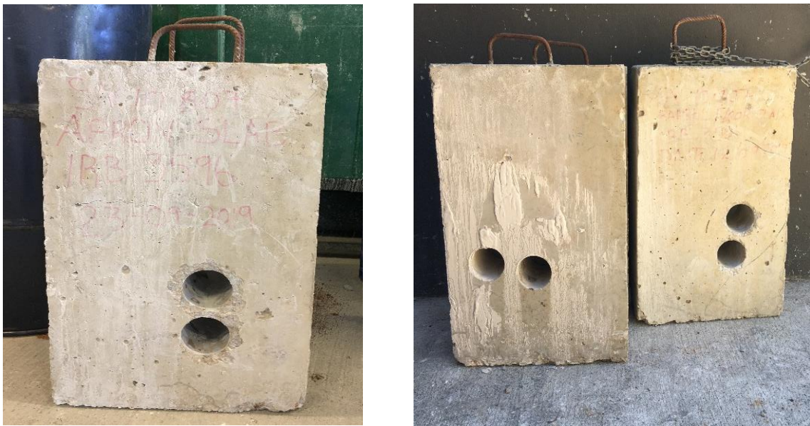
Figure 3-2: N2 road expansion panels of (0.7m X 0.45m X 0.15 m) used as a source of recycled fine aggregates
