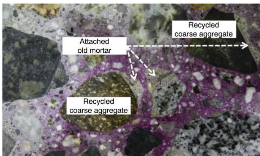
Figure 2-13: An illustration of the recycled concrete aggregate interface under microscopic investigation by (Seo & Choi, 2014)
