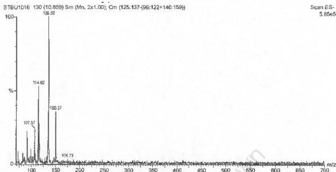
Figure 2-21. Mass spectrum of 4-vinylguaiacol (10) produced from the 1 mM reaction of ferulic acid with immobilised laccase in aqueous media.
