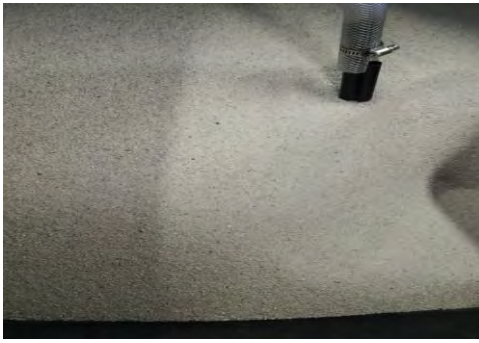
Figure 3.18: sandblasting sand with feed hose
