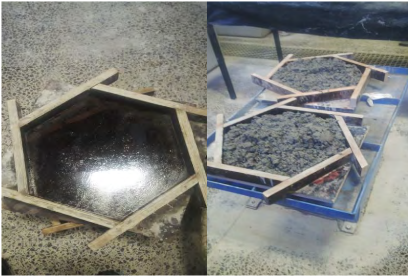
Figure 3.12: prepared mould and concrete filled moulds to be vibrated
