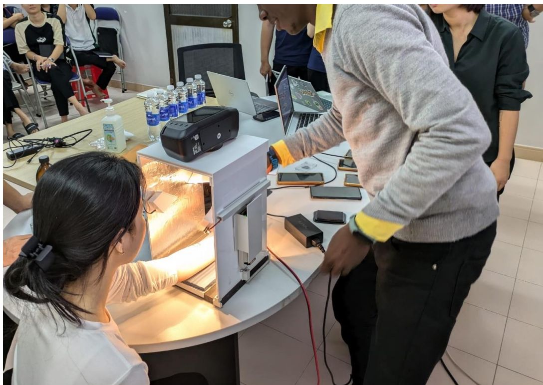
Figure 4.1: Picture showing the acquisition of hypercubes of TST indurations at the study site in Vietnam.
