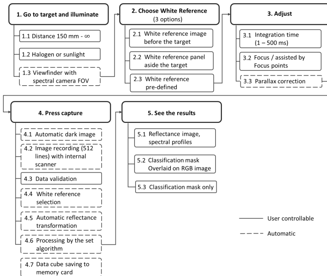
Figure 3.1: Revisiting the imaging protocol for spectral signature acquisition using the Specim IQ HSI camera (Behmann et al., 2018).
