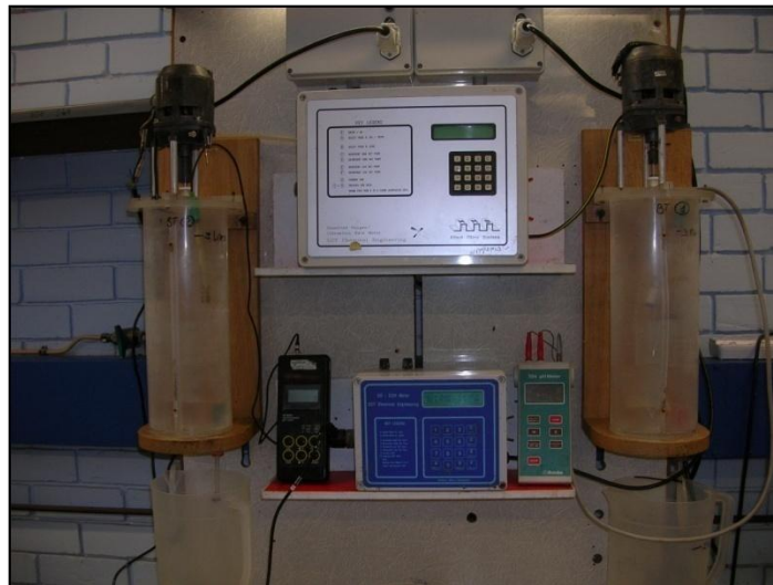
Figure IV.10: Batch reactors set up for nitrification and aerobic batch tests. Also shown are the OUR boxes for oxygen measurement as well as the pH meters.
