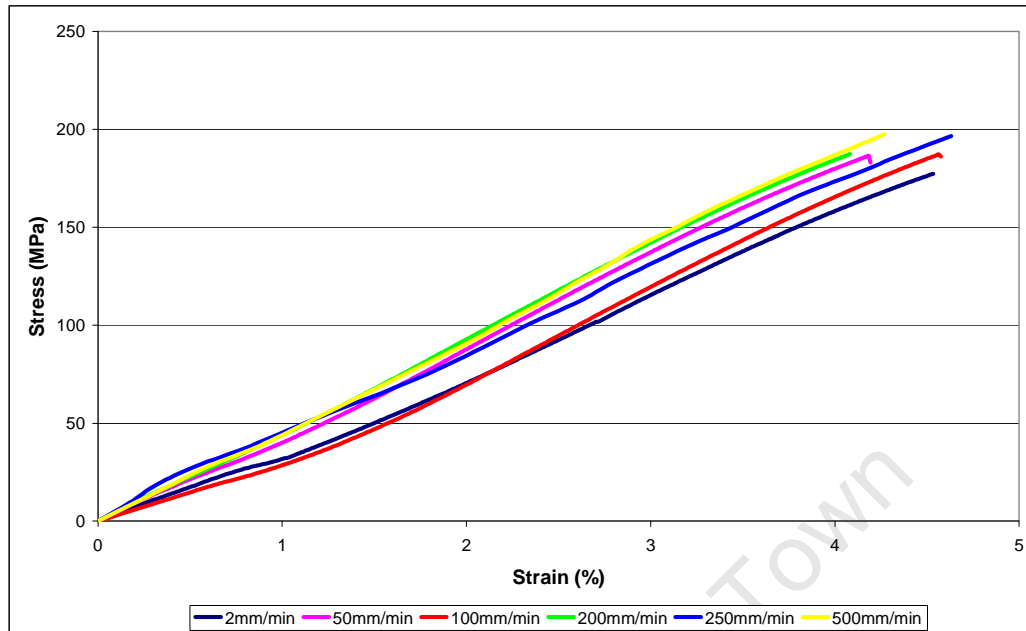
Figure 4.14: Stress-strain curves for 40% GF PPS composite at room temperature and different test speeds.
