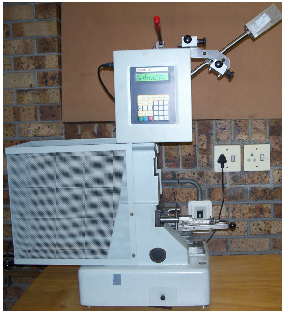
Figure 3.7: The Zwick/Roell impact tester for Izod and Charpy impact testing.
