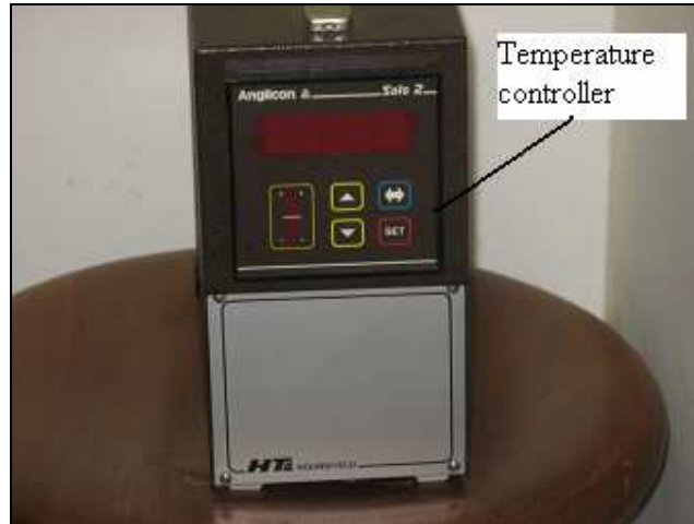
Figure 3.5: The temperature controller connected to the Hounsfield tensile tester.
