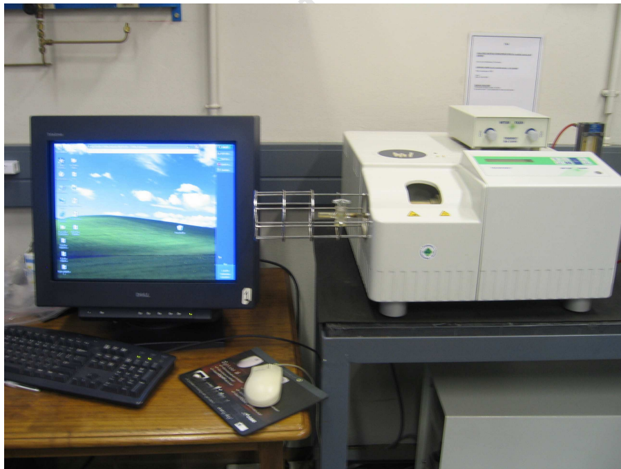
Figure 3.1: The Metlar Toledo SDTA 851 thermogravimetric analyser used for the TGA tests of the PPS resin.
