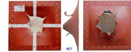
#07 Group 3b, NEC 30g PE4 on 3mm panel OD = 3mm, Face Down at 1,5m
