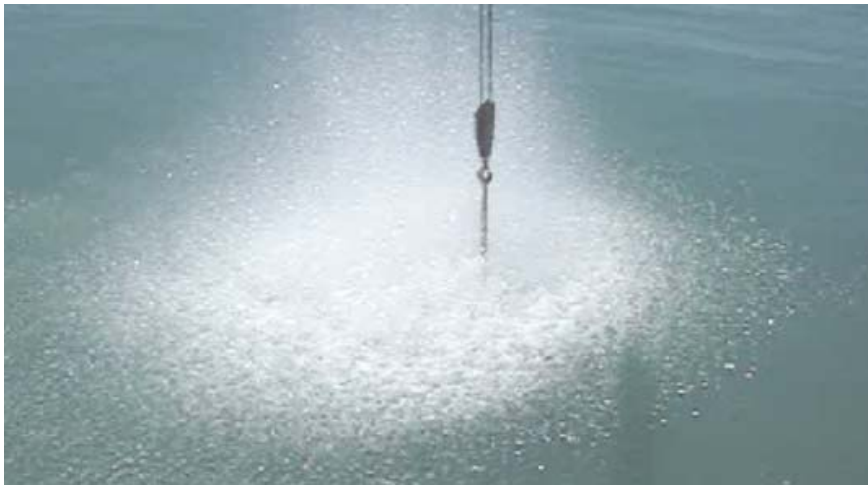
Figure 4-10 : Surface effects due to reflected shock wave
