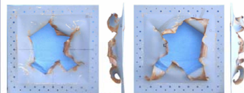
#1212 Group 4. NEC 30g PE4 on 1,2mm panel OD = 12mm, Orientation Face Down at 1,5m
