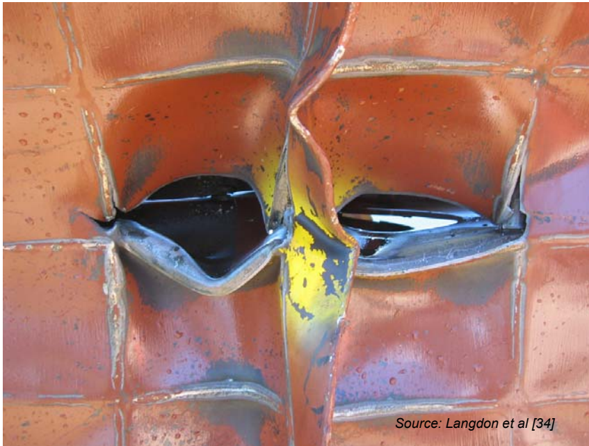
Figure 2-6: Tearing along stiffeners on an air backed target
