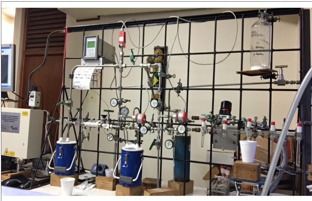
Figure 4.1: Laser Fluorination system in the Stable Isotopes Lab with Laser, traps, kBr trap, sample bottles, etc (Department of Geological sciences UCT).
