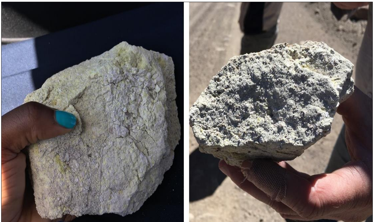
Figure 3.8: Sulfur rich altered rock from Cabanas mine (left) and a sulfur rich altered dacite from Ollagüe (right).
