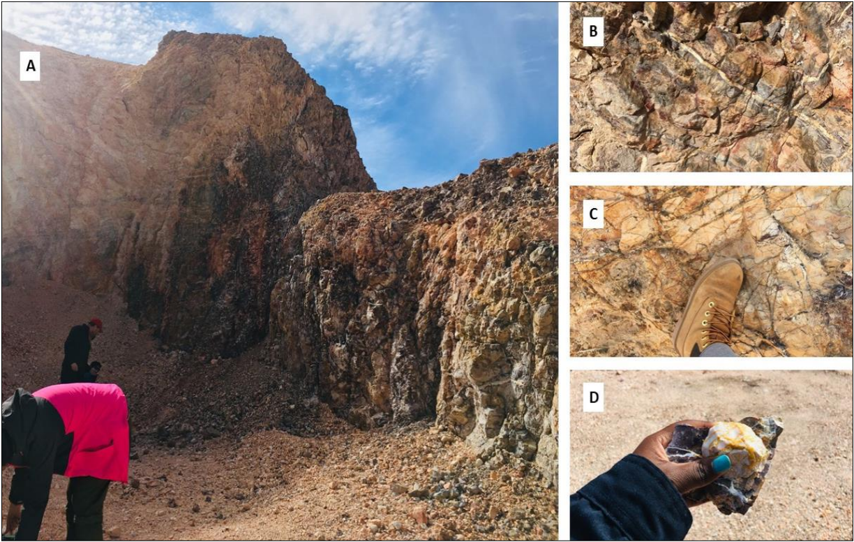
Figure 3.9: A view of the mined out mineralized zone (A). Frame (B) and (C) show the brecciated outcrops with a lot of veins. Frame (D) shows the opaline rock with shades of purple, white and yellow.
