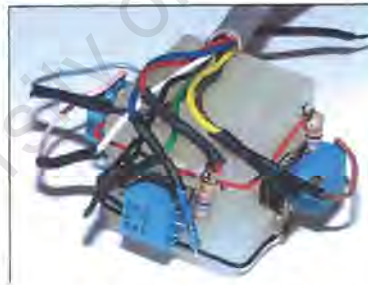
Figure 4.8: The three accelerometers mounted orthogonally on the nylon block
