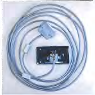
Figure 4.9: The shielding of the accelerometers
