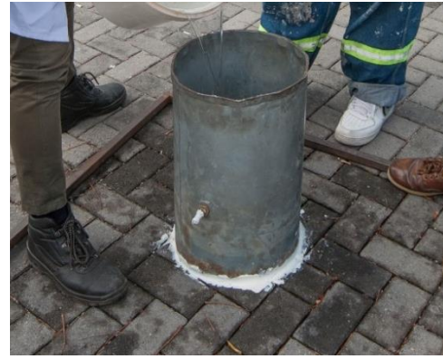
(b) ASTM C1781 test apparatus
