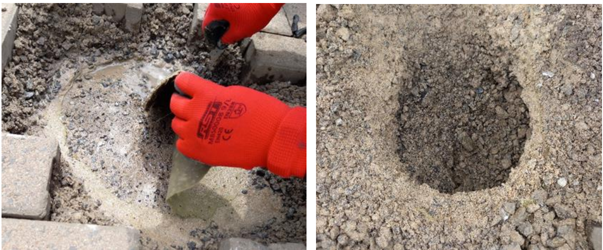
Figure E-5: Type IV clogging (in the base courses)
