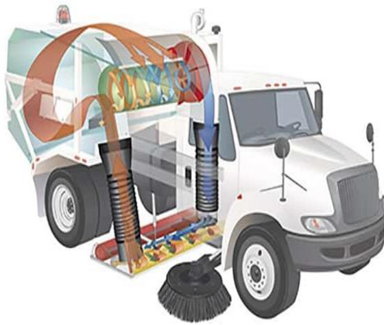
(a) Street sweeping mechanism
