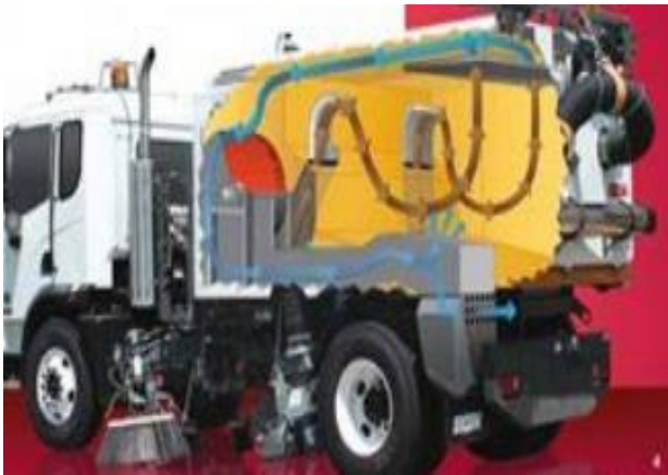
(a) Vacuum-based street sweeping mechanism
