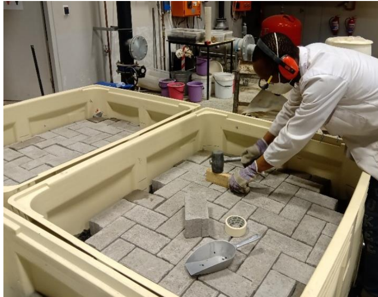
Figure 5-5: Pavers being installed in the experimental cells
