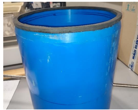
(b) Mod-ASTM C1781 test apparatus underside
