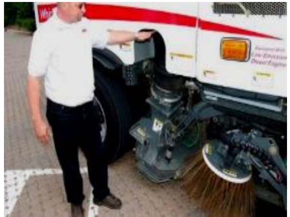
(b) Rotating windrow broom 'close up'
