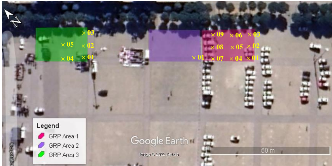
Figure 4-54: GRP infiltration test spots (Map source: Google Earth Pro, 2022)
