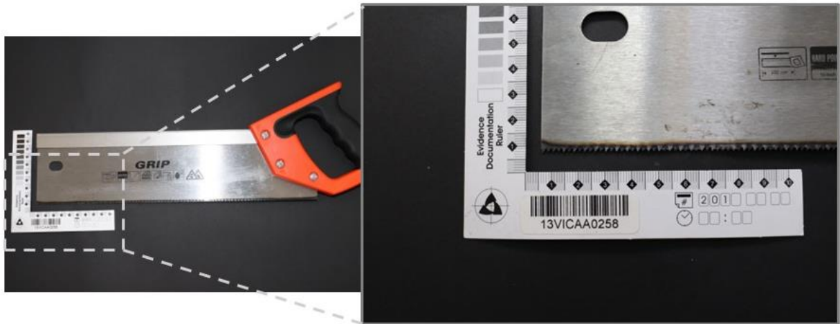
Figure 1: 13 TPI backsaw used in the study.
