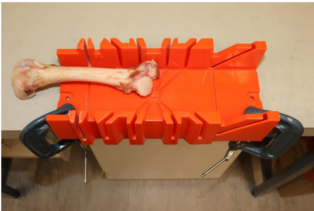
Figure 2: Mitre block secured with G-clamps.
