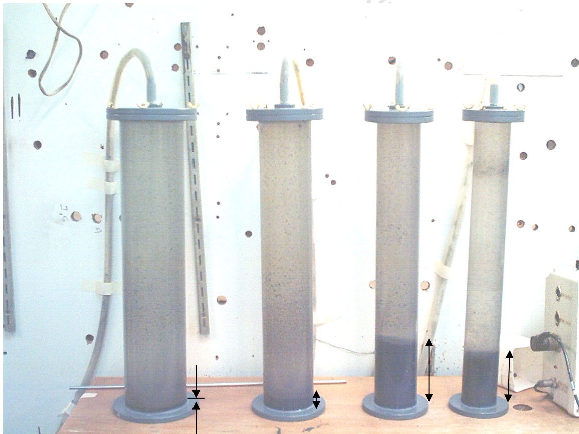
Figure 6.10: Picture of the settleometer showing R1 sludge fraction retained in each column at steady state ( Q = 10.17 L/h and V_{up} = 1.16 m/h in the largest column).
