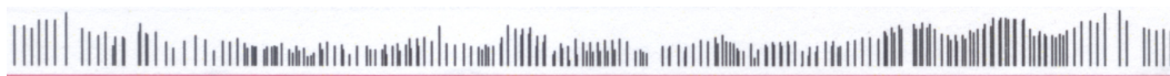
Figure 2-6. Enlargement of a portion of the conductivity graph on a Barcode summary for Mzinto Dam from 1994 to 2006: the maximum conductivity is about 40\text{mS.m}^{-1} . Between 1995 and 2005, the Department of Water Affairs and Forestry and Umgeni Water were both regularly monitoring the same site (on different days). The two interleaved data sets are clearly visible, but the duplication only became apparent when the Umgeni Water data were imported into DWAF's database in 2006.
