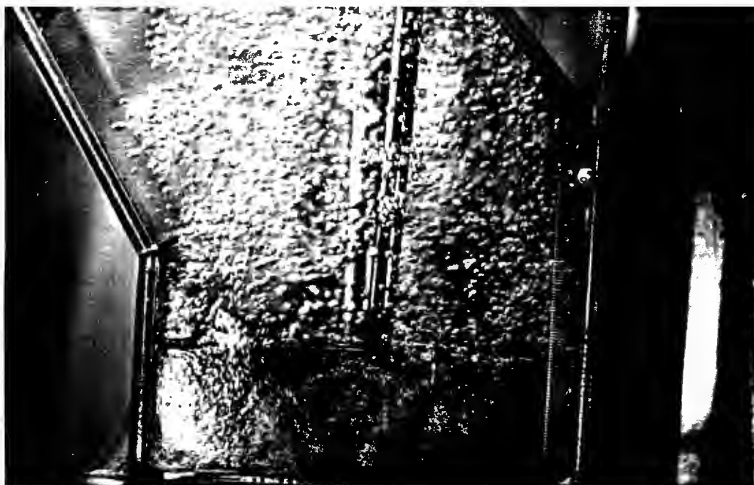
Figure 4.3 : Bubbles produced in the batch flotation cell in the absence of any reagents. Aeration rate was 4 \text{ l.min}^{-1} and impeller speed 1200 rpm.
