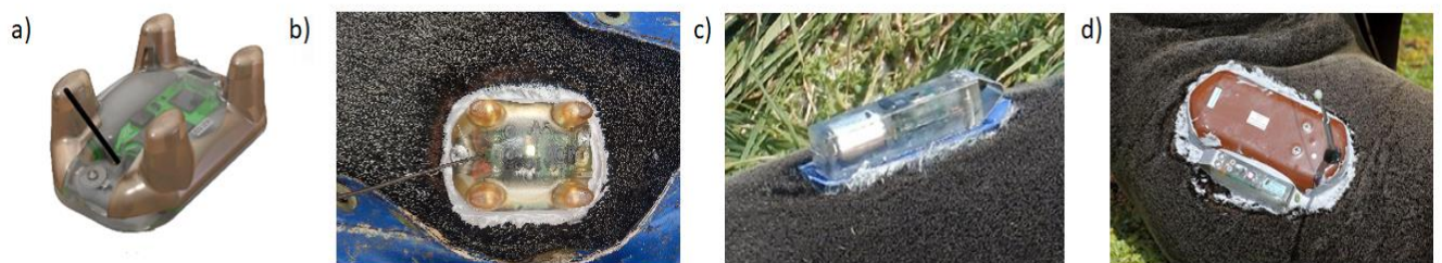
Figure 2.2: A schematic of Wildlife Computers' SPLASH 10-351 tag (a) (Adapted from Wildlife Computers' product feature sheets) attached to a subantarctic fur seal (b) at Marion Island and a Wildlife Computers' TDR-MK9 (c) alongside a PTT tag (d). Pictures (b) and (c) were taken by Sean Evans, while (d) was taken
