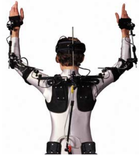
(a) Gypsy mechanical MOCAP system. Image from [75]
