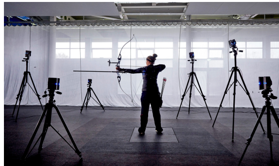
(b) Vicon passive marker-based MOCAP system. Image from [58].
