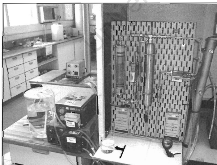
Figure 3-3: The gas flow set-up used to introduce the gas mixture of sulfur dioxide and oxygen. Peristaltic pumps and a water bath are situated to the left of the gas flow equipment.
