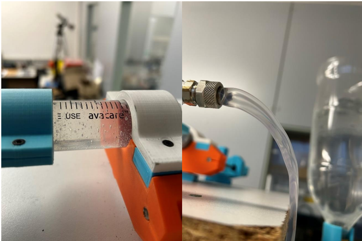
Figure 38: Void formation in the pump and the flexible tubing "ribboning" in the gel syringe pump.
