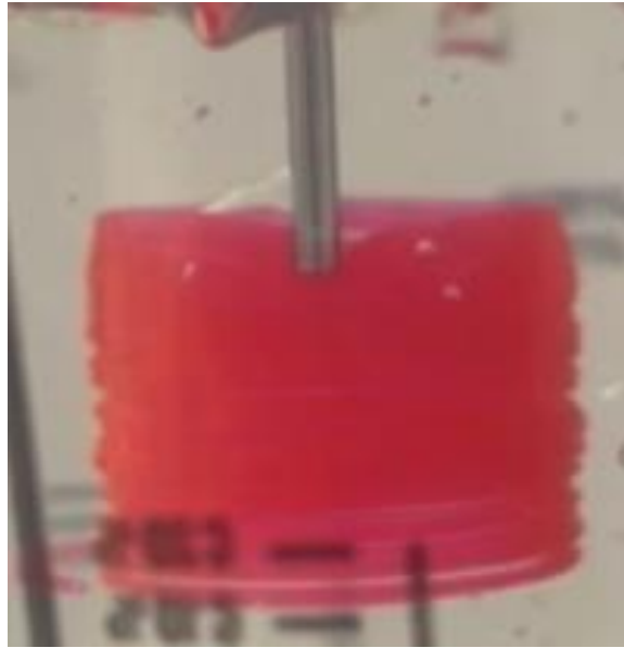
Figure 56: The wake behind the needle draws up material just printed and then forces that material down again when it next passes.
