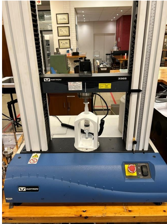
Figure 62: The stand and syringe set up in the loading apparatus.
