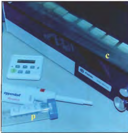
Figure 6.5. The Fisher® slide warmer had a perspex cover so that a pale cloud (c) of moisture formed over the smears and moisture loss was minimised. If evaporation of the pepsin (p) during the warming had been marked, additional reagent was applied after five minutes.
