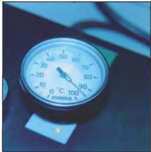
Figure 6.8. The temperature of the Fisher® heating block was monitored with a Reuger® surface thermometer. The sensor of the thermometer was placed on a glass slide (s) to obtain an accurate indication of the temperature attained by the slides being heated.
