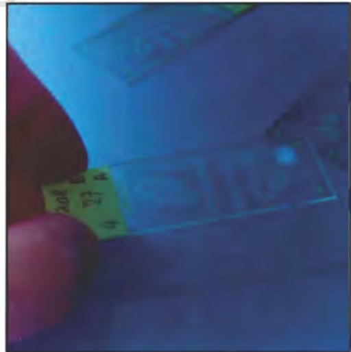
Figure 6.4. Two sectors or "work areas" slightly larger than the size of a 18 x 18 mm cover slip were demarcated on each slide using a wax Pen. ®
