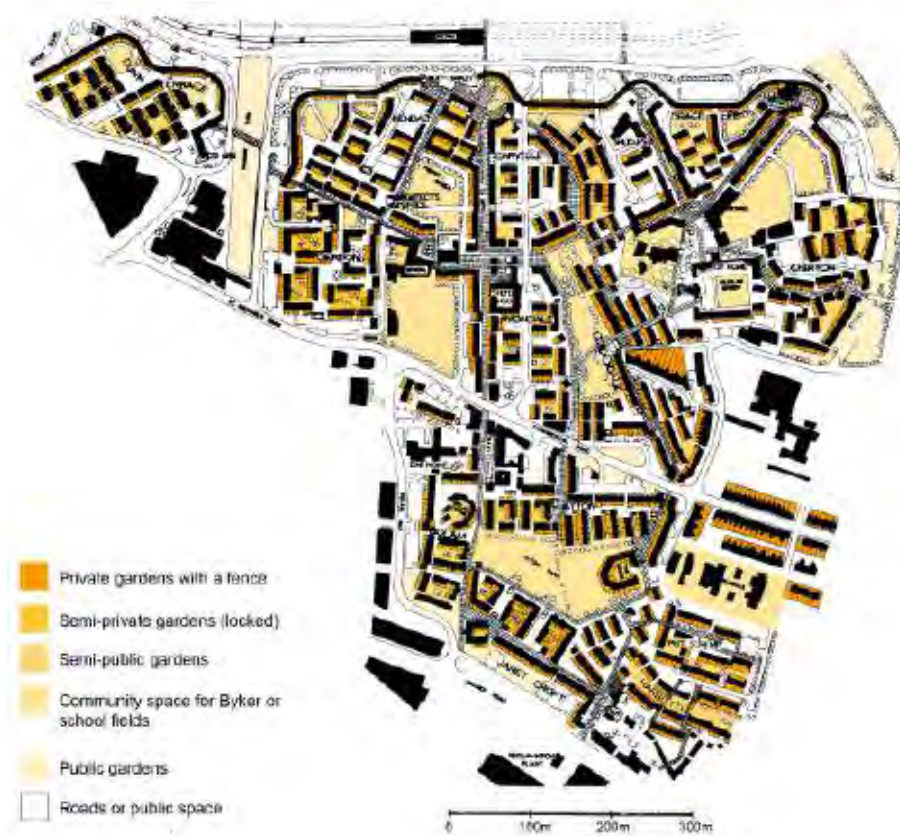
Figure 10: This urban plan of Byker shows the hierarchy of open space. The project has a great range of open space from private gardens to cordoned-off semi-private gardens to community space for the project. (Image adapted from - Harvard University Graduate School of Design, 1988: 15)
