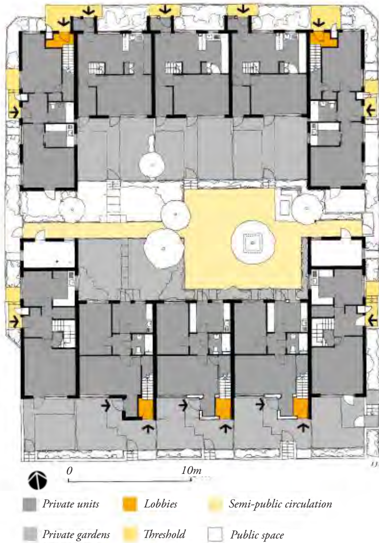
Figure 12: Kendal block in the Byker project. This block has a range of units in a perimeter block. Steps, lobbies or private gardens give a threshold to the units. In the centre of the block is a semi-private garden for these units to use. (Adapted from - Harvard University Graduate School of Design, 1988)
