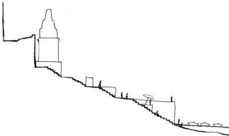
Figure 57: Section through the ghats embankment. Stone piers lead off the wider platform to create a viewing space.
