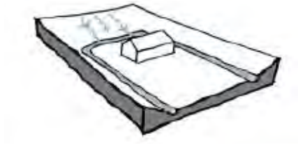
Figure 51: A diagram showing how swales can direct water away from buildings to avoid water damage. (Drawing based off: Schultz, 2013)
